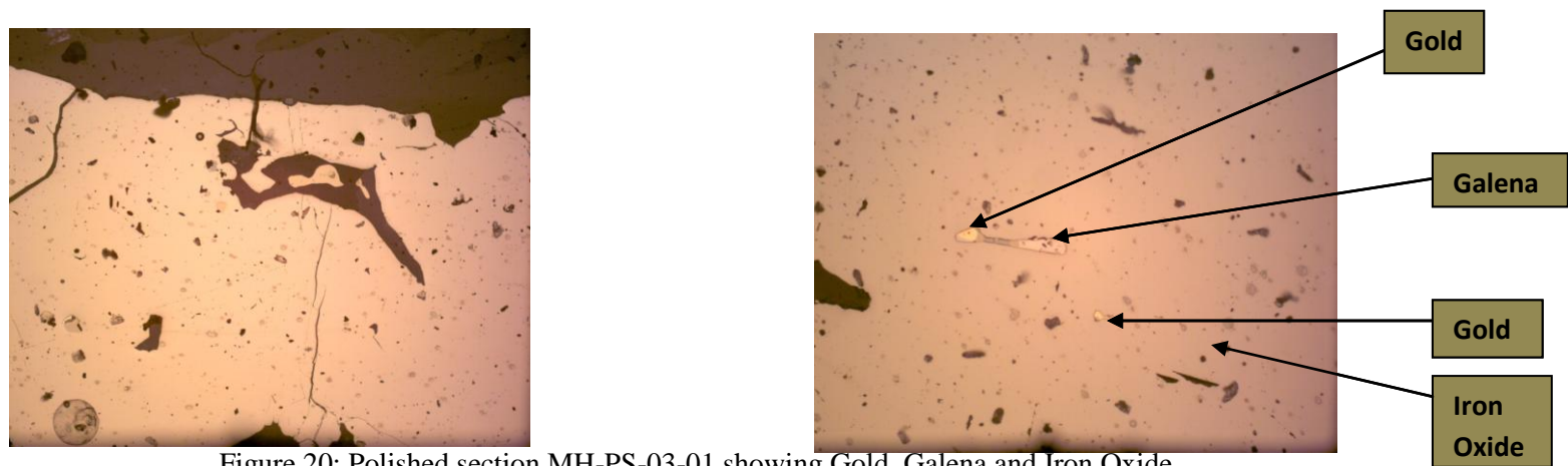
Figure 20: Polished section MH-PS-03-01 showing Gold, Galena and Iron Oxide
