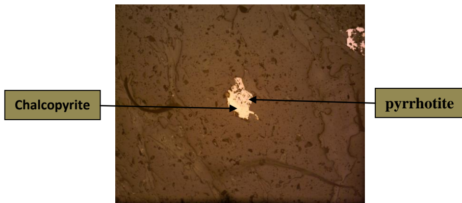
Figure 34 : Polished section MH-TS-21-01 showing Pyrrhotite and Chalcopyrite
