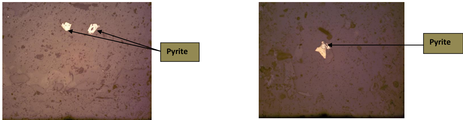
Figure 24: Polished section MH-TS-5-03 showing Pyrite
