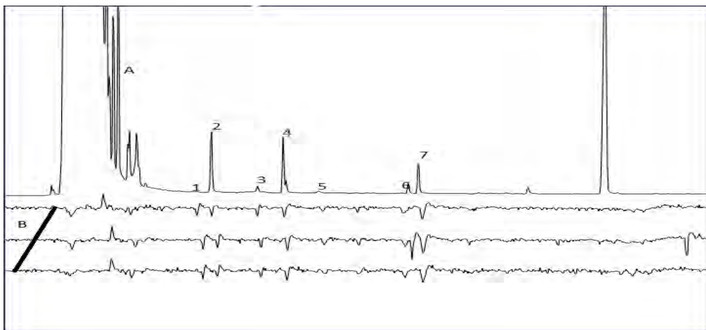
Figure. 6 EAD chromatograph of female B. zonata . Top trace (A) represents the FID response, the bottom trace (B) the antennal response. Peak numbers correspond to compounds in Table 2.
