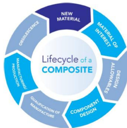
Figure 2.3 Typical lifecycle of a composite [7]
