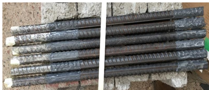
Figure 3-5: Deformed bars after application of non-corrosive epoxy
