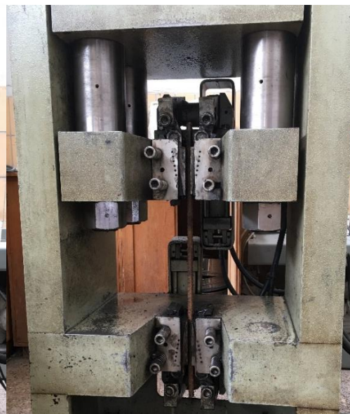
Figure 3-2 Test of the Deformed rebar
