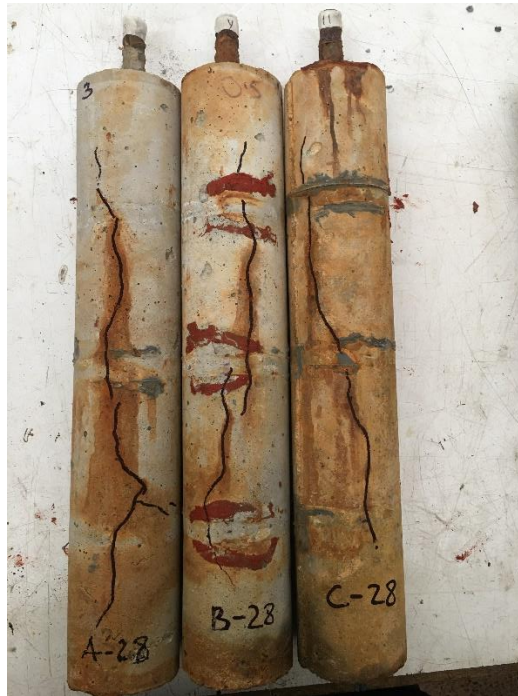
Figure 4-12: Crack pattern of the samples
