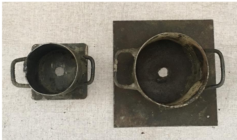
Figure 3-9: The bases of the formworks and their central hole
