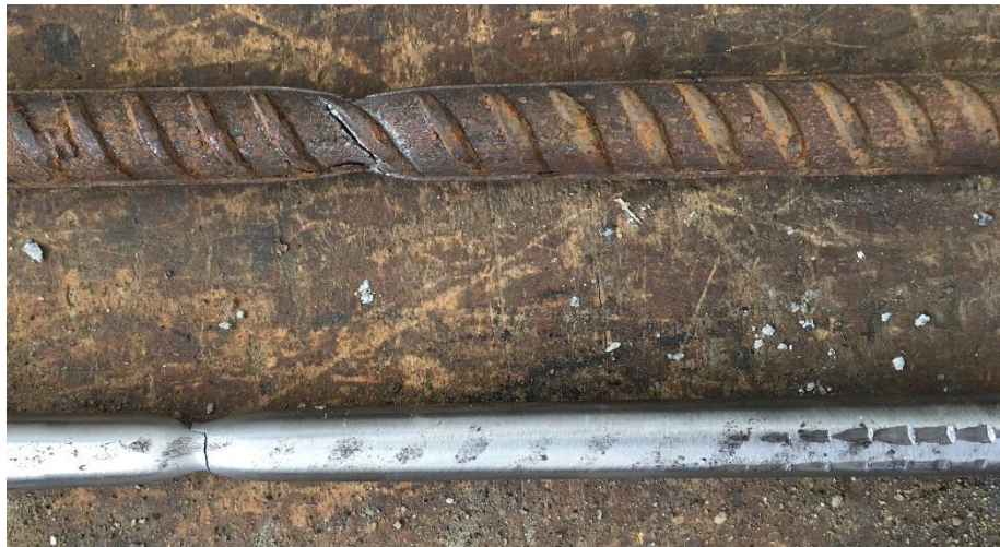
Figure 3-3: Rebar Samples after rupture
