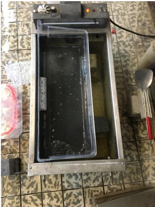
Figure 3-21: Rebars soaked in the solution
