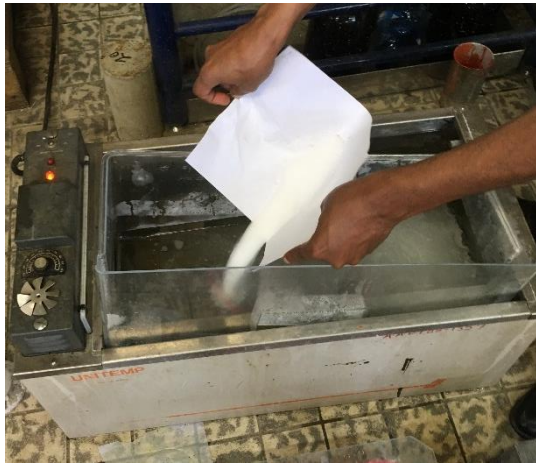
Figure 3-20: Preparation of the solution for cleaning the corrosion products
