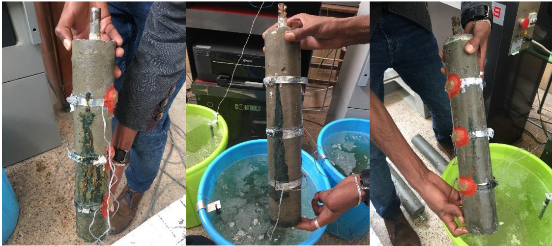
Figure 4-2: Samples after the completion of ACT (AP-28, A-28 and C-28 respectively)
