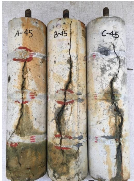
Figure 4-16: Crack pattern of the samples
