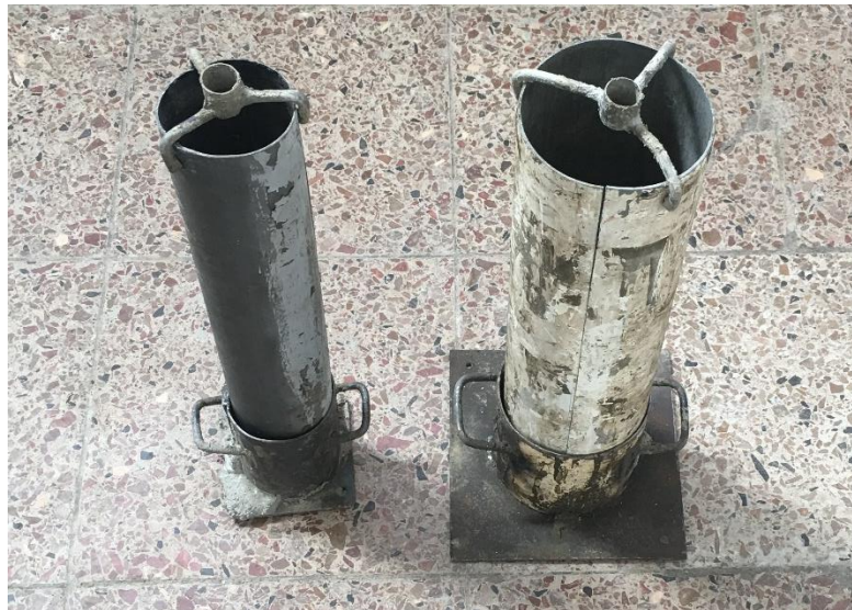
Figure 3-7: Formworks used in preparing the samples
