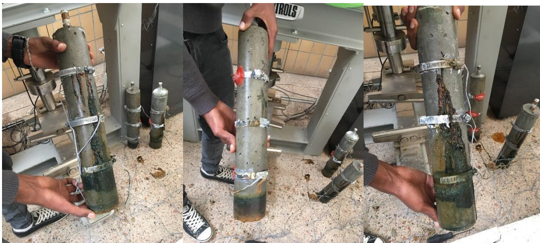
Figure 4-7: Samples after the completion of ACT (B-28, BP-28 and CP-28 respectively)
