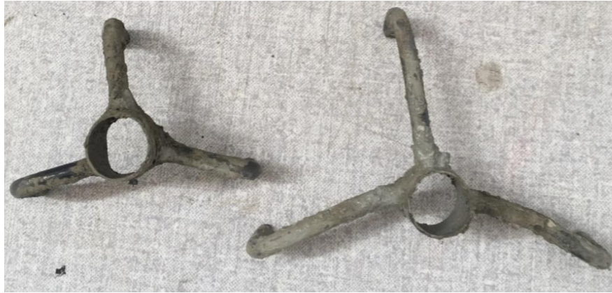
Figure 3-8: Tripod like metal used to keep the rebar at the center
