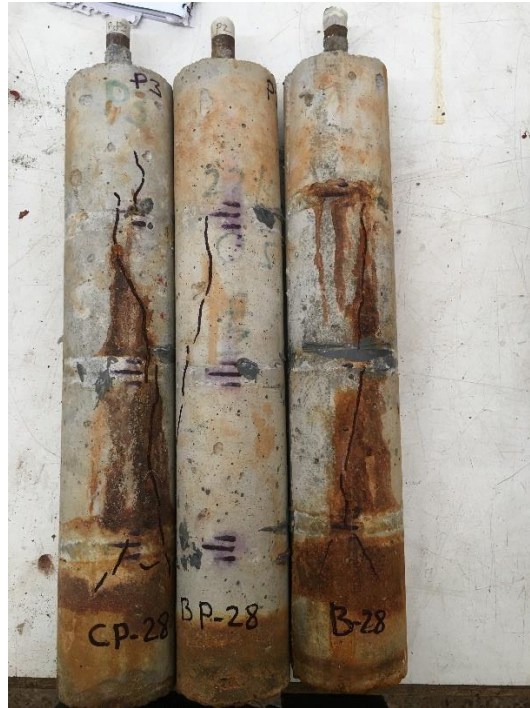
Figure 4-8: Crack pattern of the samples
