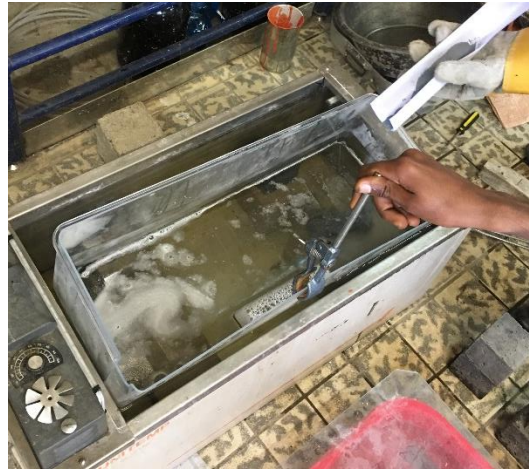
Figure 3-20: Preparation of the solution for cleaning the corrosion products
