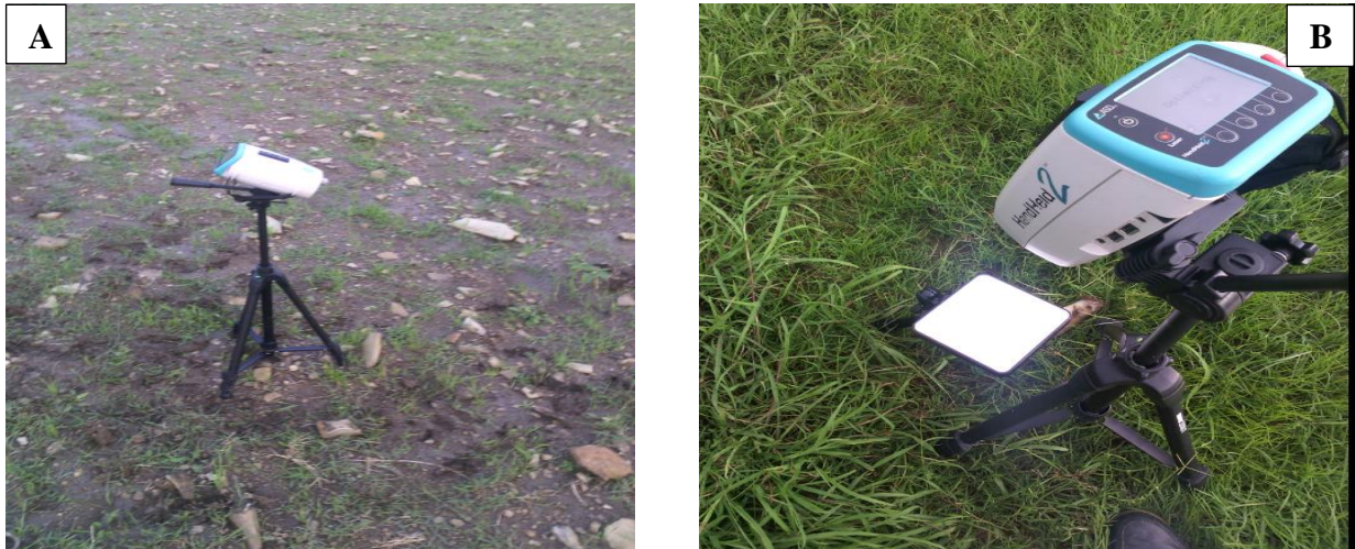
Fig.28: Photo during the field survey of reflectance from different land uses in Upper Tekeze using the Spectroradiometer. Photo in A and B were examples for bare soil and vegetation cover types respectively
