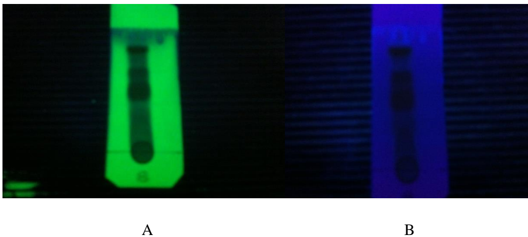
Figure 4: Thin Layer Chromatography profile of butanol fraction of Hypericum revolutum at 254 nm (A) and 366 nm (B)
