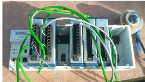
Figure 3-6: Photograph of NI cDAQ-9172 data acquisition system used in this study
