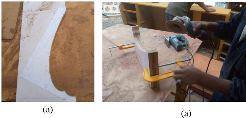
Figure 5-1: Photograph of (a) wooden pattern and (b) gridding the rough edges
