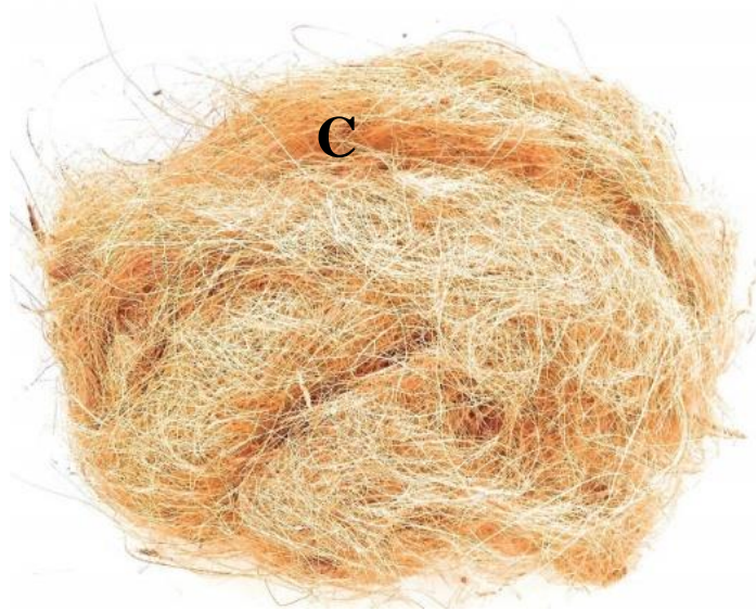
Figure 2. 7: a) Aspen pad, b) palash fiber pad and c) coconut fiber.
