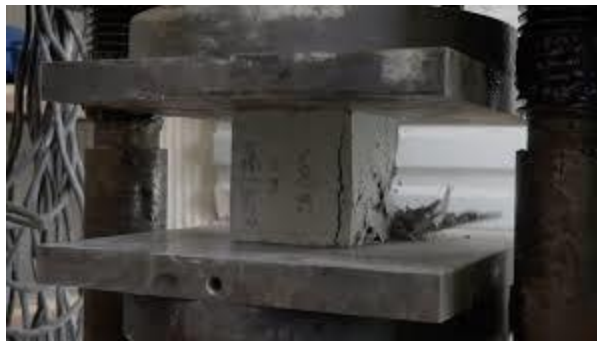
Figure 3-2 Cube Testing Under Compression Machine
