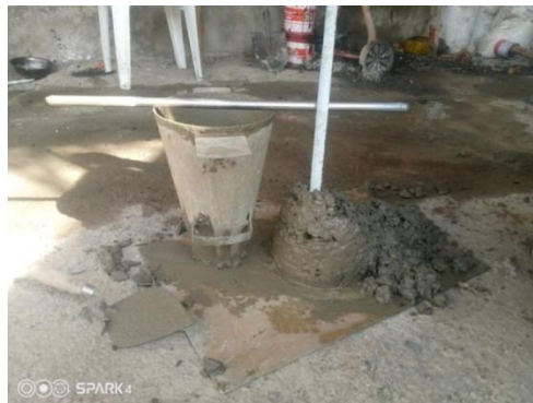
Figure 3-1 Slump Test Equipment & Procedure Illustration
