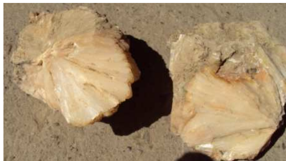
Figure 7: Picture of natural stilbite rock sample from Ethiopian
