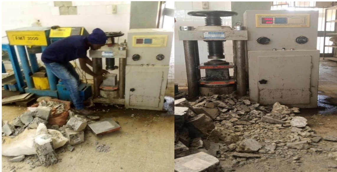
Figure 4.6 compressive strength machine and tested cubic concrete
