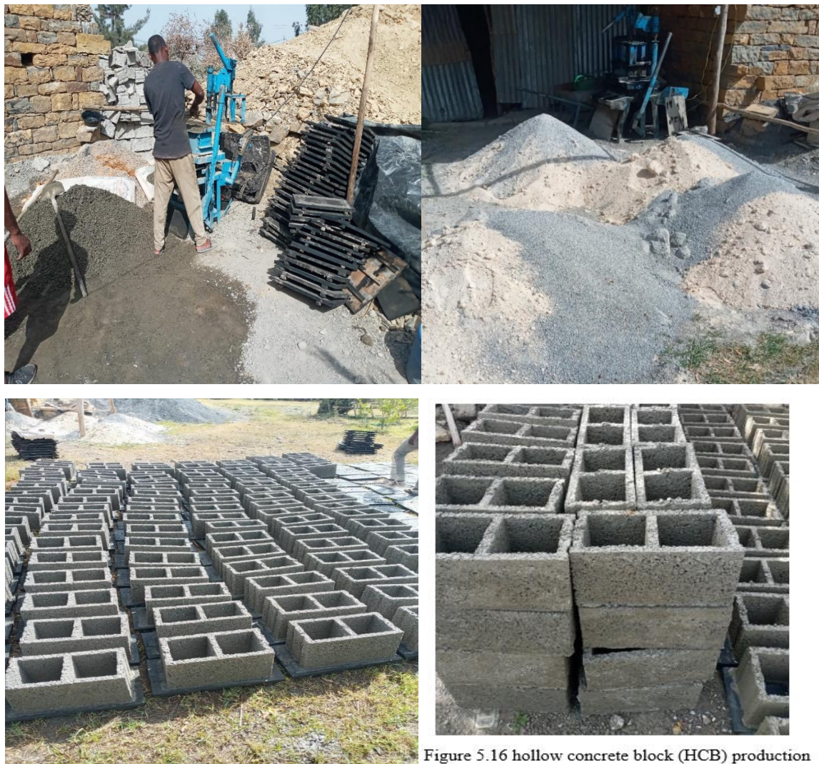
Figure 4.10 Hollow concrete block production site
