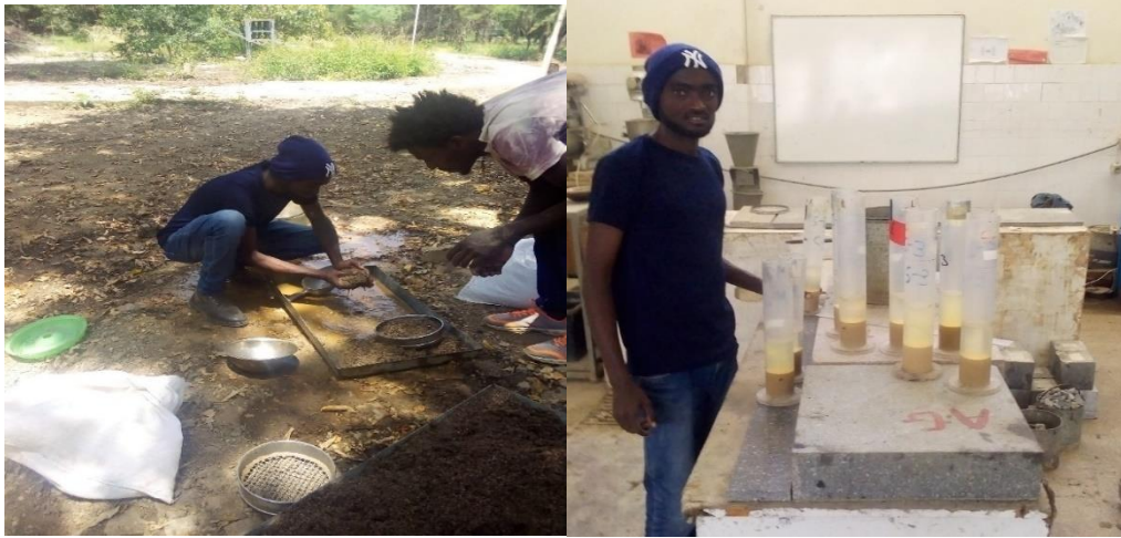
Figure 4.3 CSS and natural (rive) sand washing
