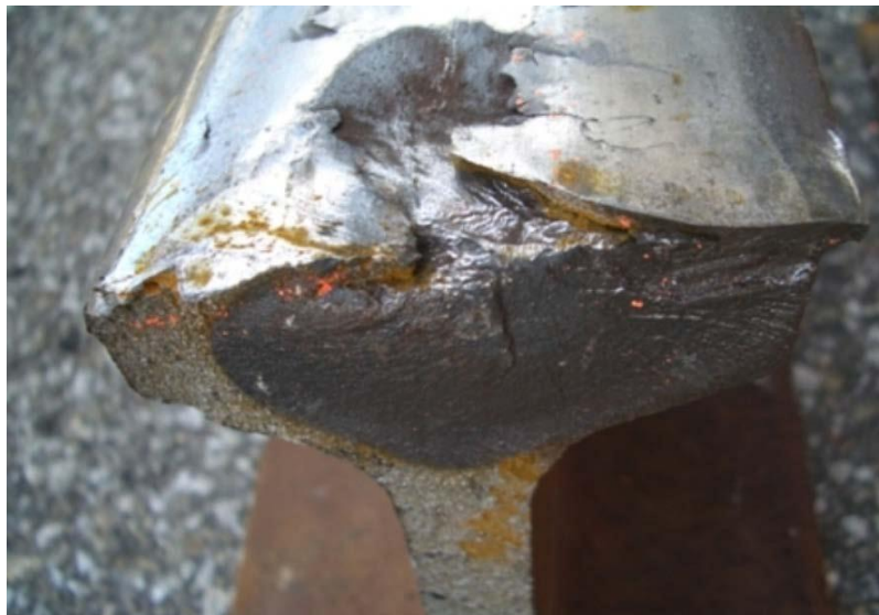
Engine Burn Fracture Showing Significant Growth
