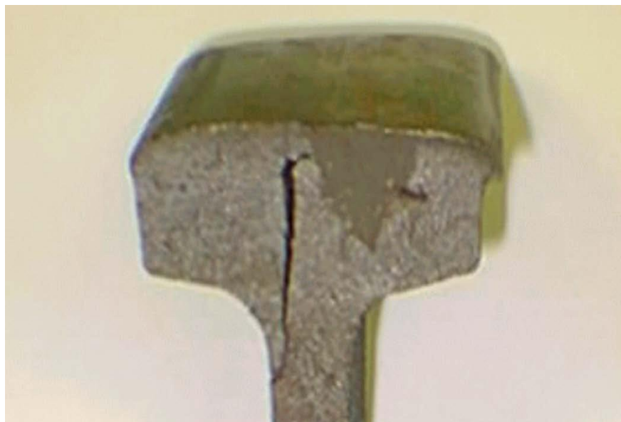
Vertical Split Head Defect Breaking out in Head/Web Fillet Area
