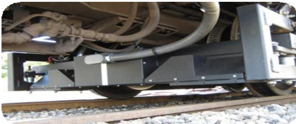
Figure 5-6 Remote Inspection Box fitted on a regular train.
