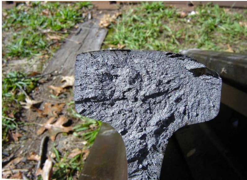
Rail Failure Fracture Face Showing No Transverse Defect
