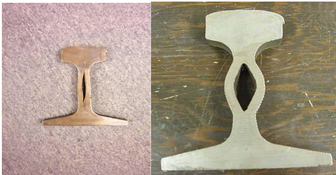
Piped Rail Showing Significant Rail Collapse
