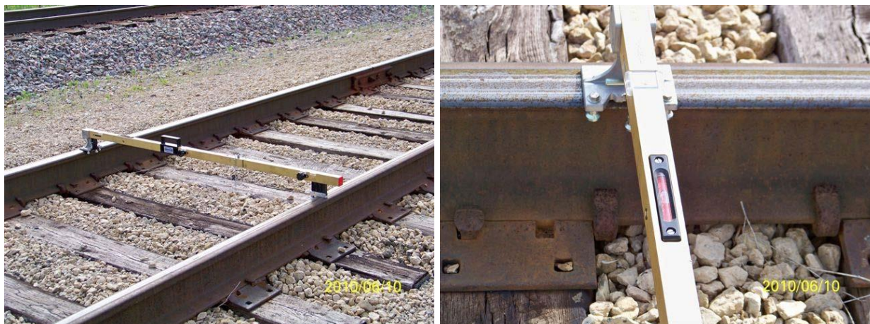
Figure 2-2 Measuring track surface deviation with a Track Level (CN 2014)
