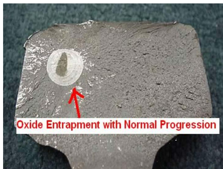
Electric Flash Butt Weld Showing Oxide Entrapment and Progression
