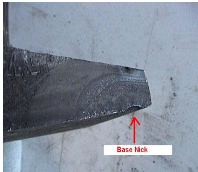
Base Fracture Showing Nick with Transverse Development
