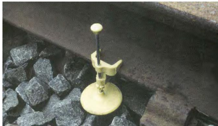
Figure 2.3.1 Showing Pell void meter fixed to bottom flange of the rail (Cope and Ellis, Calla C., 2003)
