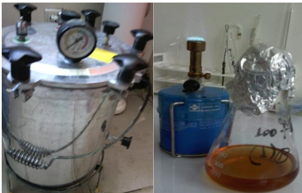
Figure 3.4: a) Sterilization machine: b) Media after sterilization
