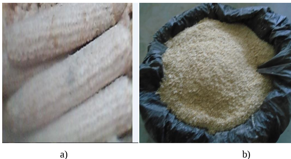
Figure 3.3 a) Corn cob sample; b) Ground sample
