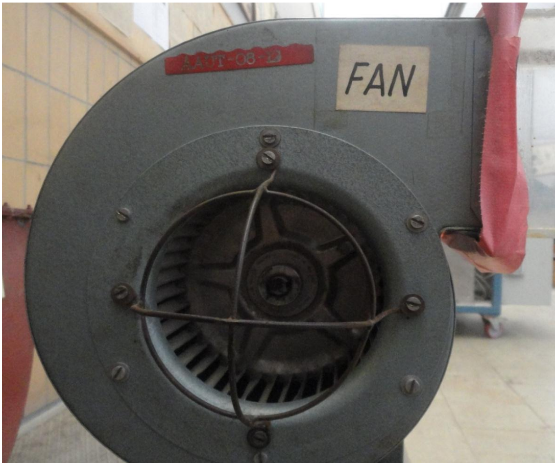
Figure 5.1: Tested forward curved centrifugal fan (the base machine)
