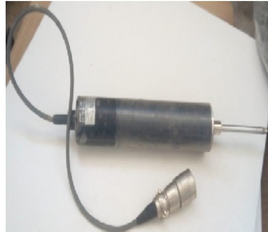
Figure 3-22 A Linear variable displacement transducer (LVDT)
