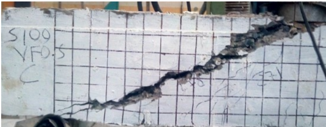
Figure 5-16 S100VF0.5%C after failure (close up view)
