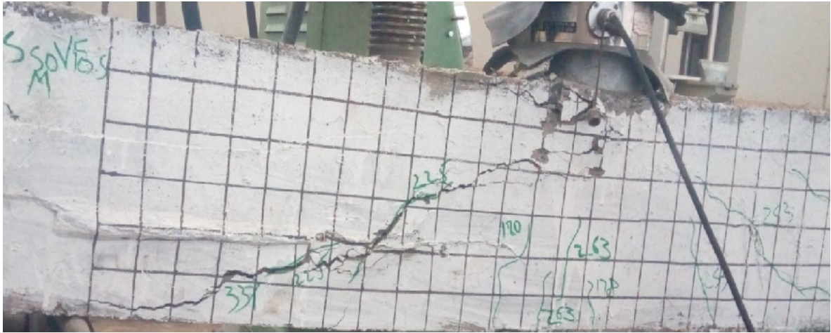
Figure 5-5 S50VF0.5%M after failure
