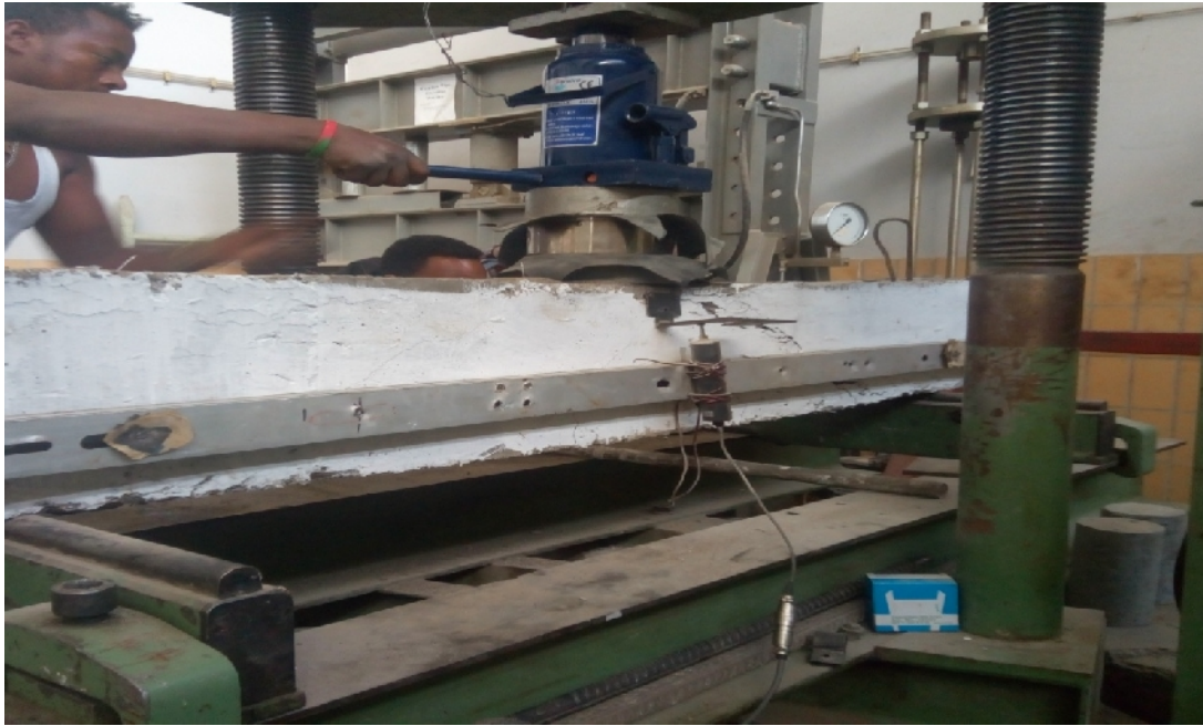
Figure 3-24 Unloading by unbolting the hydraulic jack
