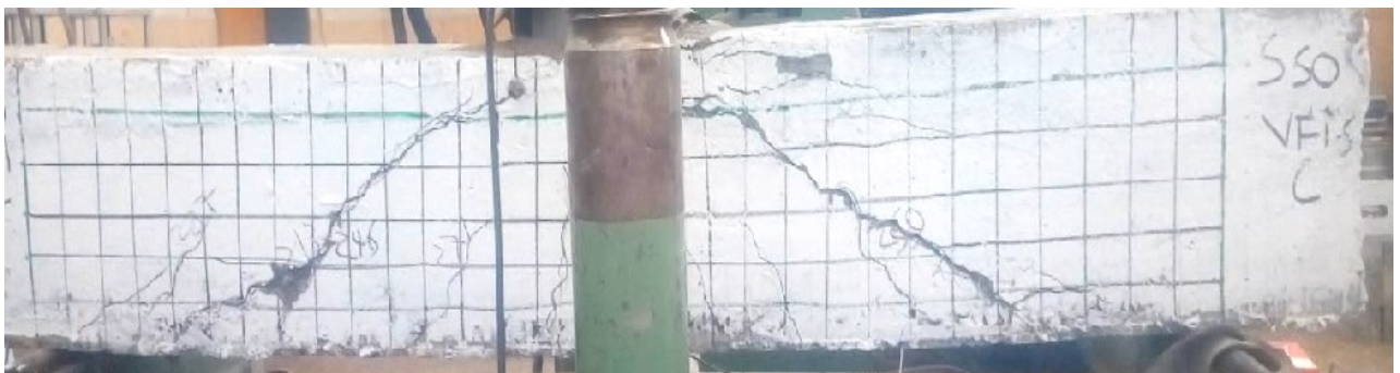
Figure 5-12 S50V1.5%C after failure
