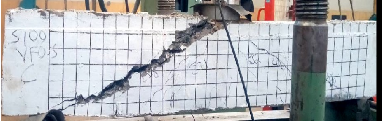
Figure 5-15 S100 VF 0.5C after failure
