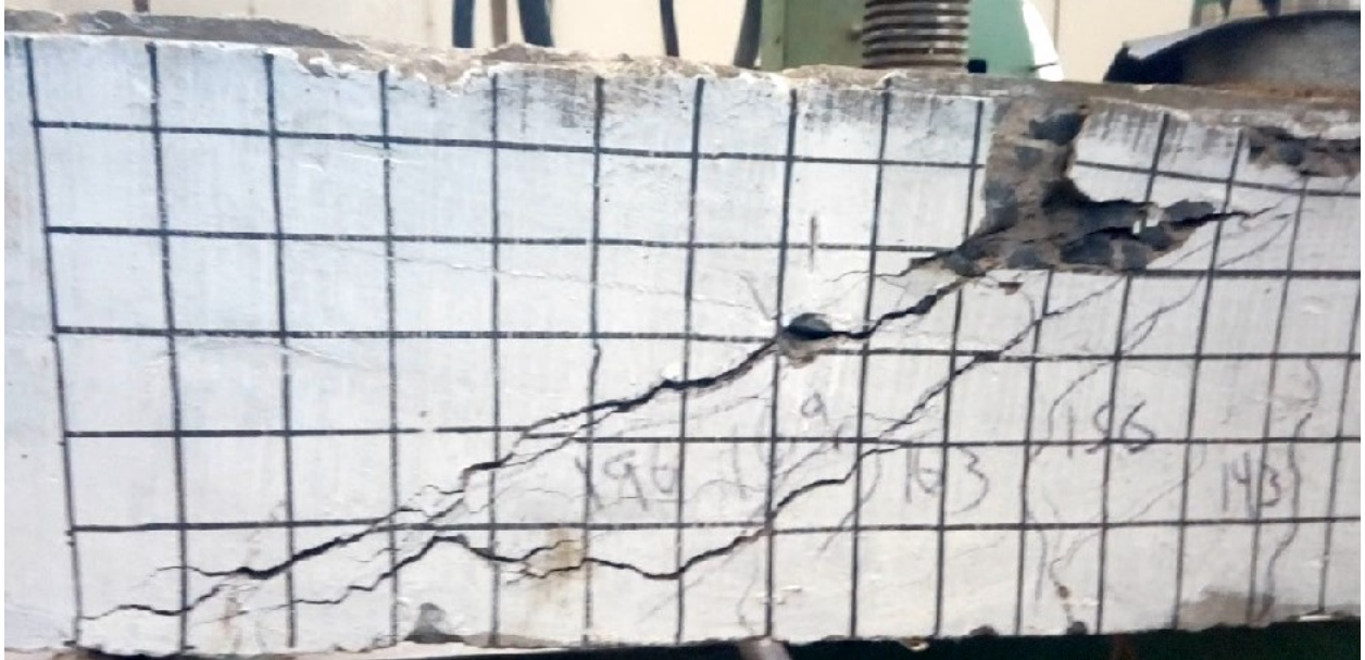
Figure 5.4 CBC after failure (close up view)
