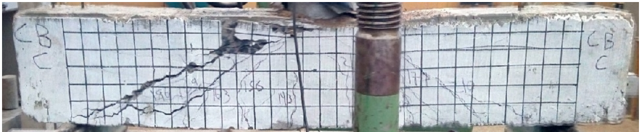
Figure 5-3 CBC after failure
