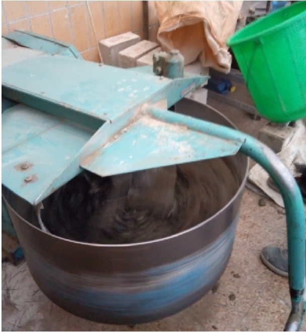
Figure 3-14 Mixing all ingredients using mixer
