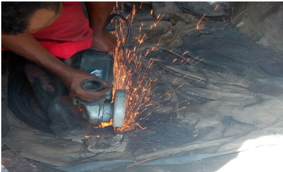
Figure 3-6 Cutting the bead wire to the required length
