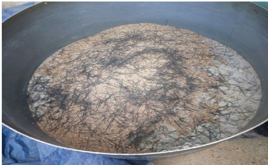
Figure 3-13 Adding steel fibers into the concrete ingredients
