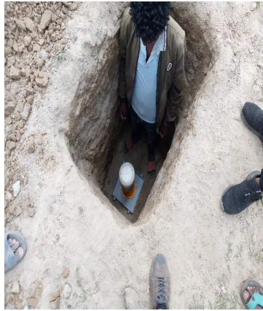
Figure 3-6: Field Density by Sand Replacement Method (on the Upper and Lower Layer)
