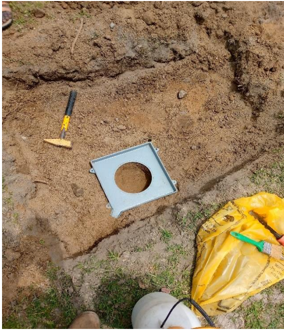
Figure 3-6: Field Density by Sand Replacement Method (on the Upper and Lower Layer)
