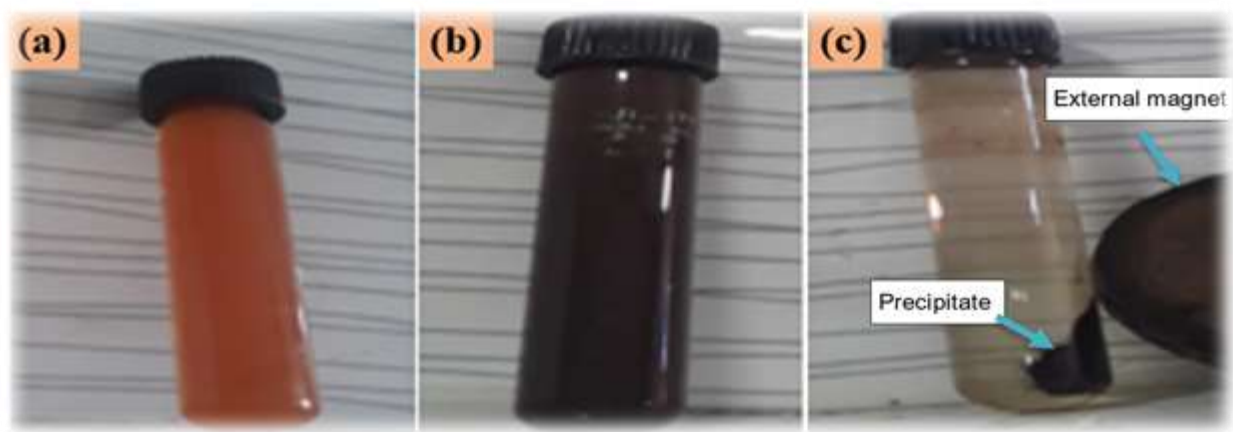
Fig.4. 2. (a) Mixtures of iron salt (b) CHE capped \text{Fe}_3\text{O}_4 -Nps Formation (c) External magnetic attraction of CHE capped \text{Fe}_3\text{O}_4 -NPs
