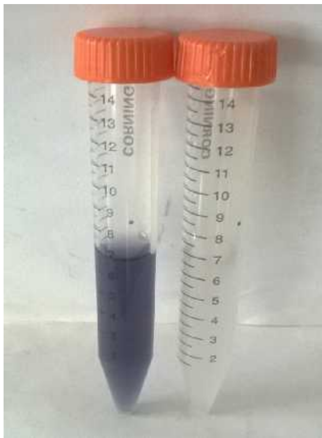
Figure 41: Tannery wastewater before (left) and after (right) treatment with R-B-3M-3 h
