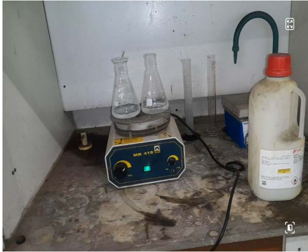
Figure 11: Water sample heated on hot plate
