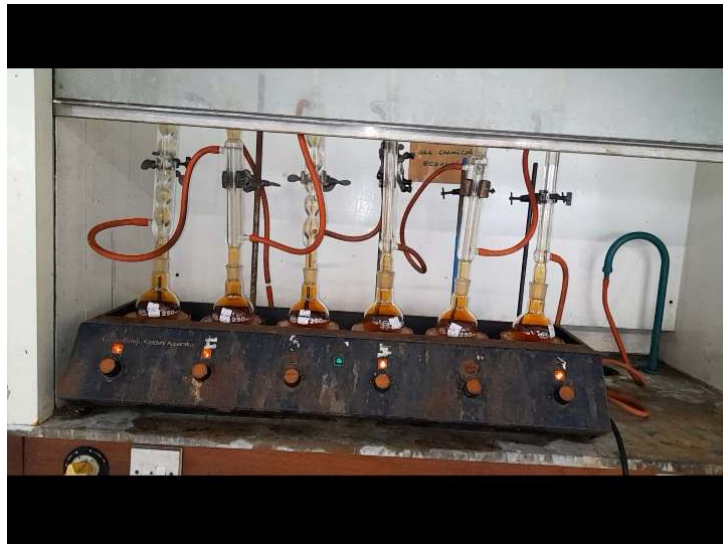
Figure 10: Soil samples heated on Kjeldhal Digestion block
