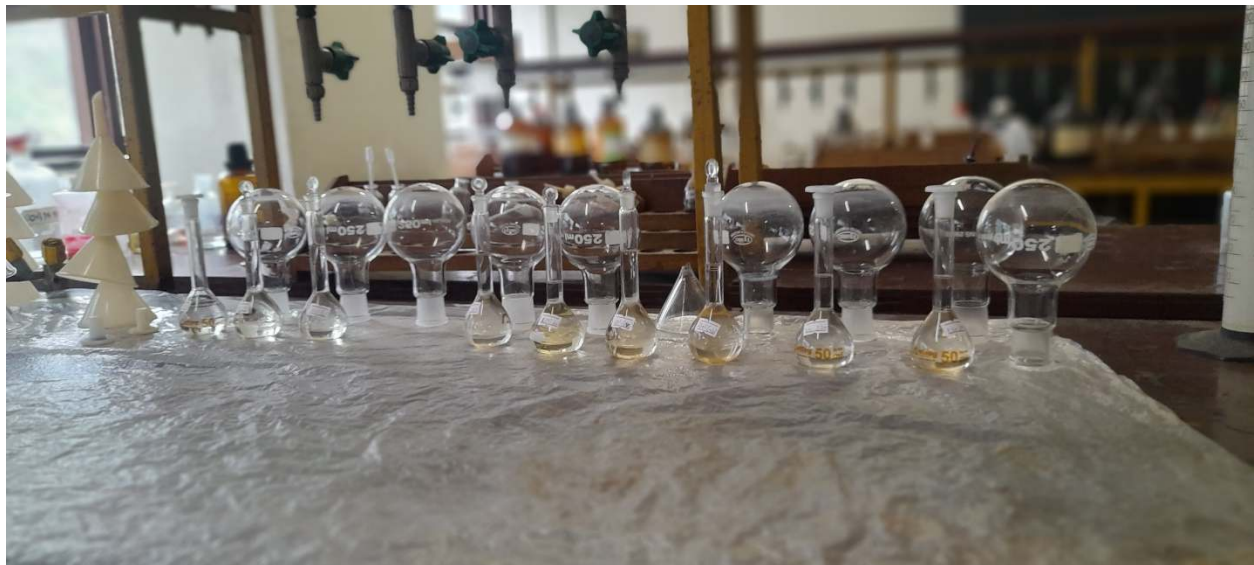
Figure 12: Samples in 50ml volumetric flask after digestion process
