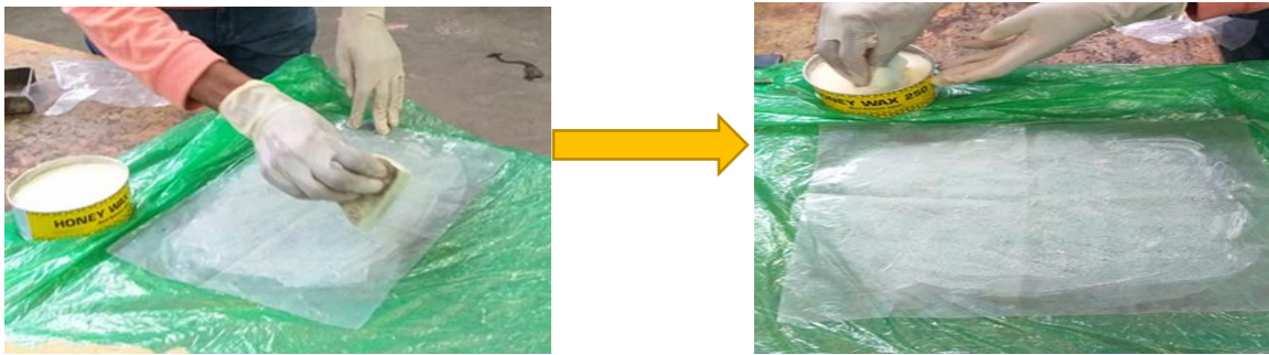
Figure 3.8: Applying wax on polyethylene plastics
