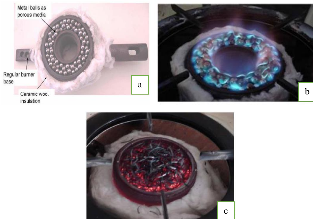
Figure 2-8 a) sealed mixing tube of a standard burner with a porous medium made of metal balls within. b) Metal ball used as porous media. C) Combustion in the porous medium of metal chips(Pantangi et al., 2007)
