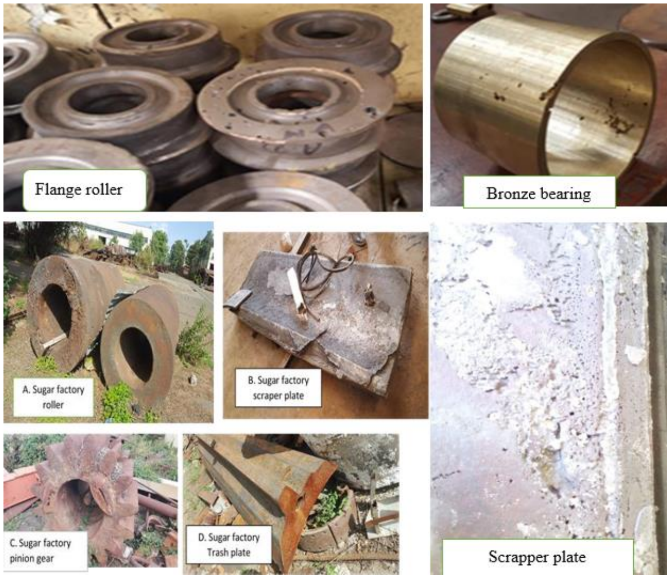
Figure 2. 2 Major casting defects on different products in Akaki Basic Metals Industry
