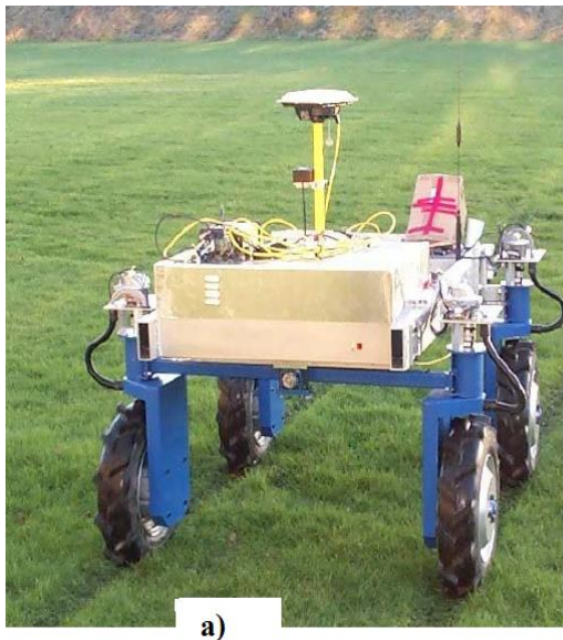
Figure 2.1 Autonomies wheeled mobile robot for: - a) weeding [8] and b) Self-guided digging and seed sowing [11]
