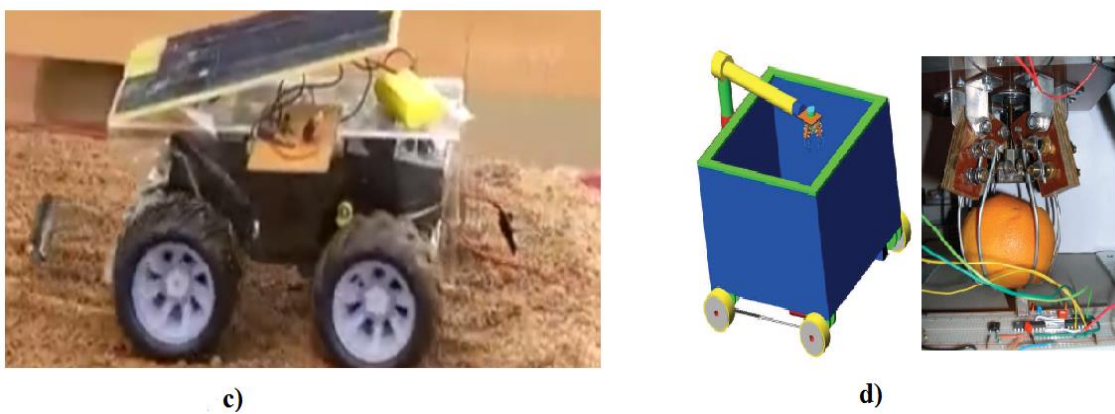
Figure 2.2 Autonomies wheeled mobile robot prototype models for c) plowing [13] and d) Suitable gripper for harvesting sensitive agricultural products [14].
