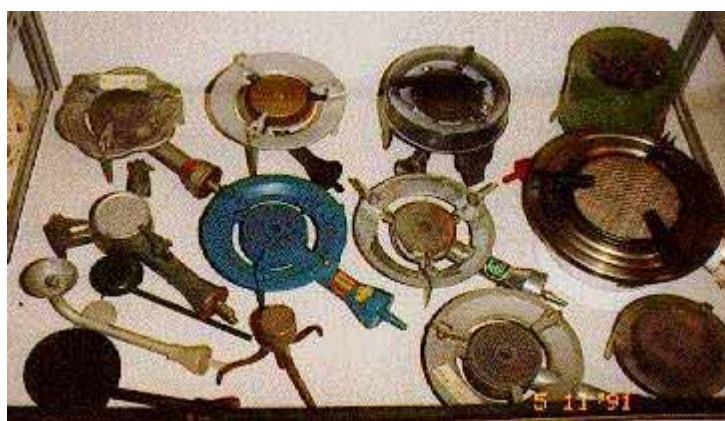
Figure 2.7: Different types of Biogas burners at an agricultural exhibition in Beijing/China
