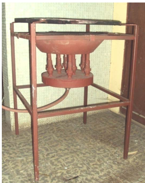
Figure 4.1: Biogas injera baking stove
