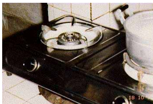
Figure 2.6: Biogas burner in china
