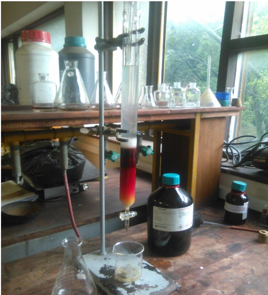
Figure 4.5: purifying methanol extract betanin by using liquid Colum chromatographic technique
