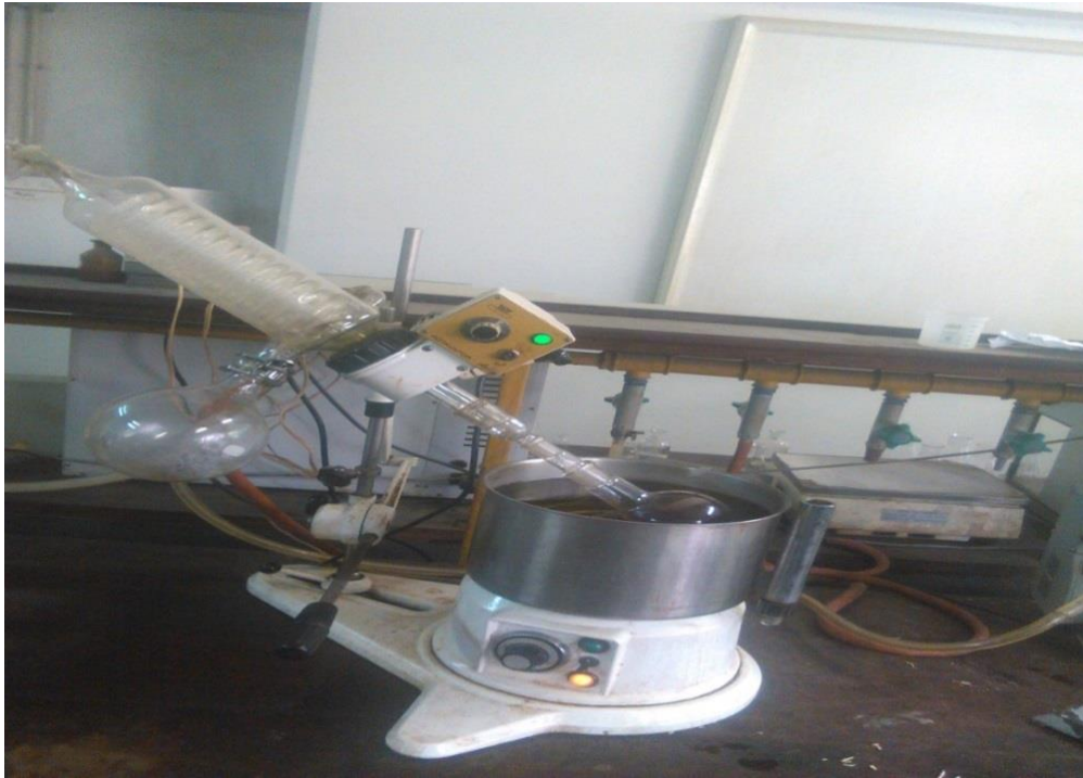
Figure 4.3: Concentrating betanin pigment by using rotary evaporator at 40 °c
