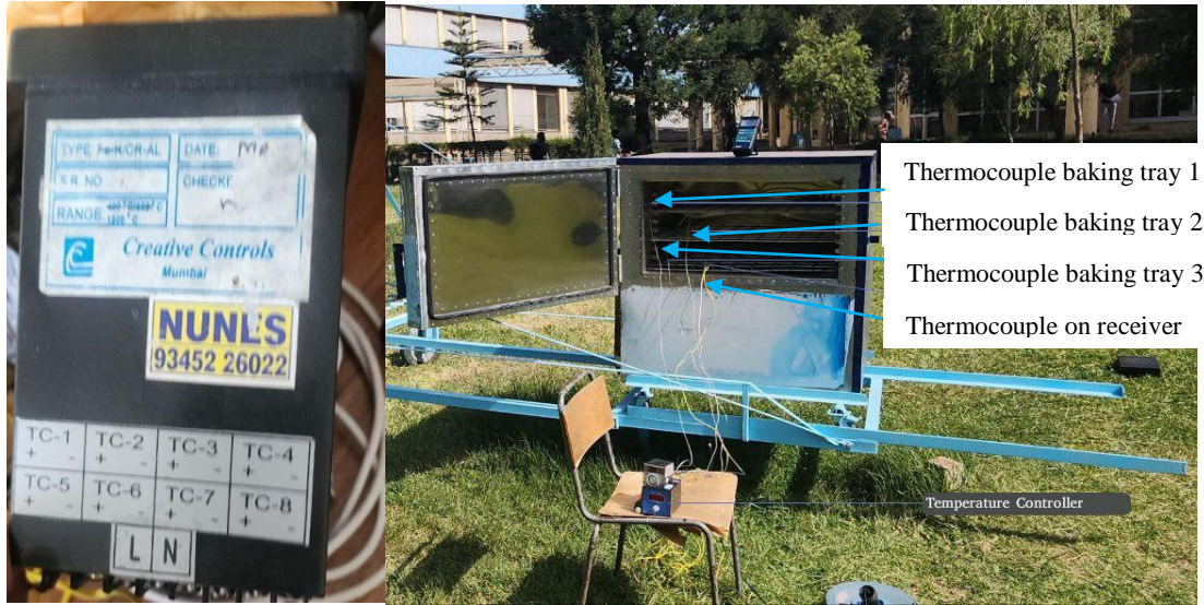
Fig. 3.5 K type thermocouples integration over different position of the solar oven
