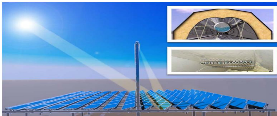
Fig. 2.21 Linear Fresnel collectors with the cavity receiver [44]
