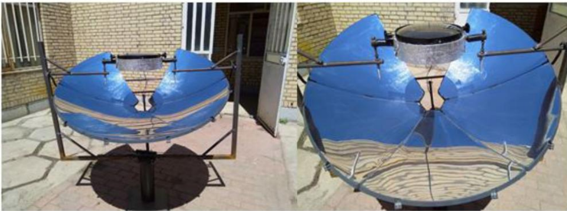
Fig. 2.11 Solar baking oven [35]
