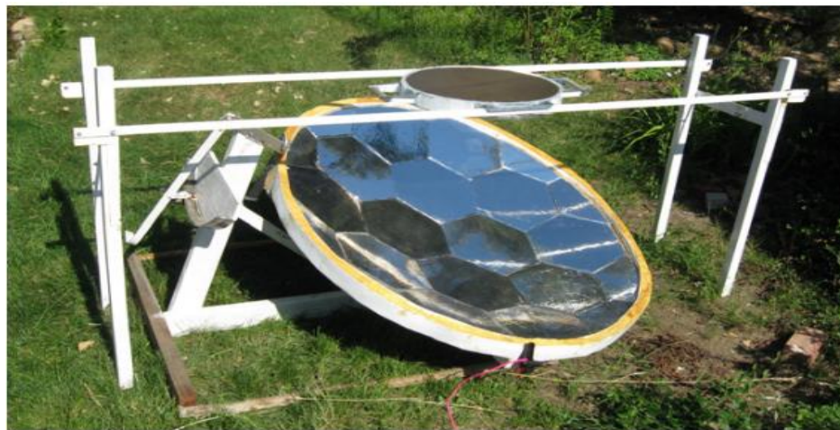
Fig. 2.10 Solar injera fryer setup [29]
