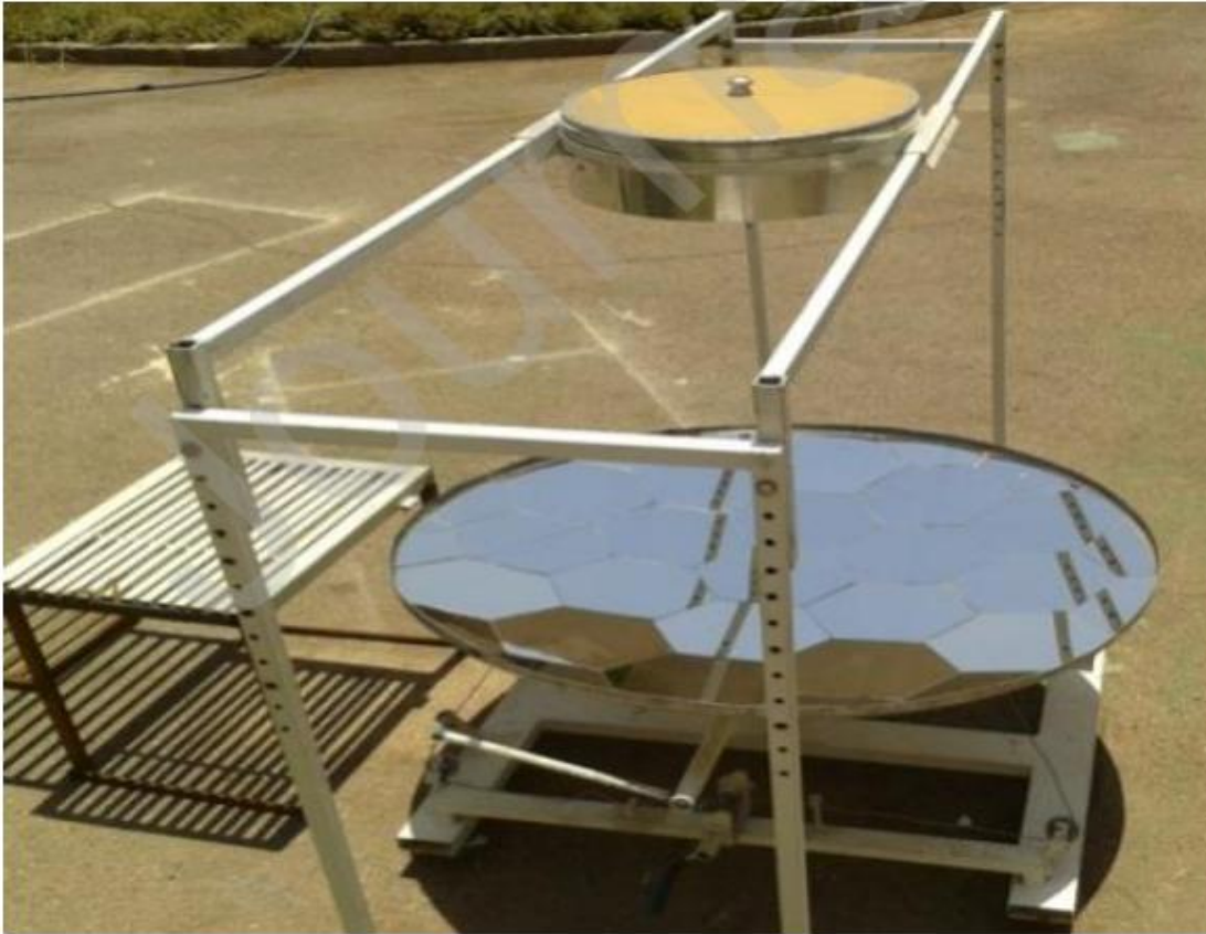
Fig. 2.13 Parabolic concentrator solar bread cooker [37]
