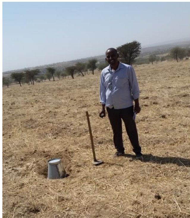
Fig. 9. 3 Single station noise measurement using TROMINO seismometer
