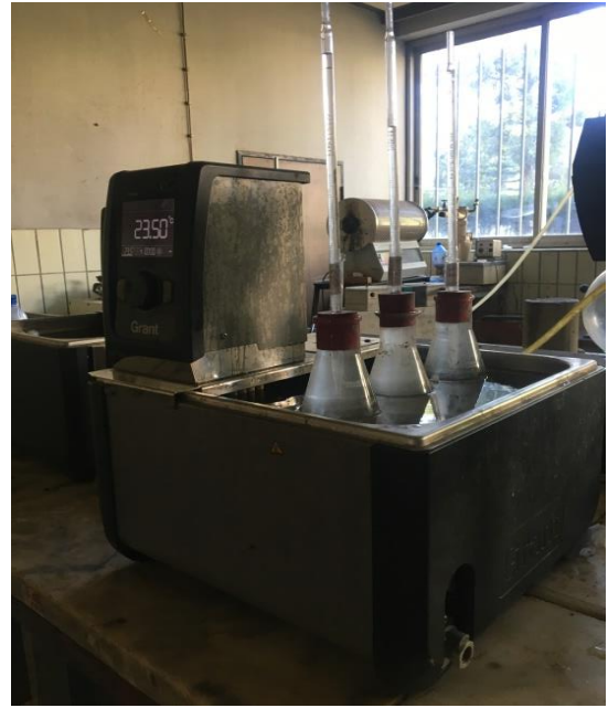
Figure 3.15 Chemical shrinkage test set up
