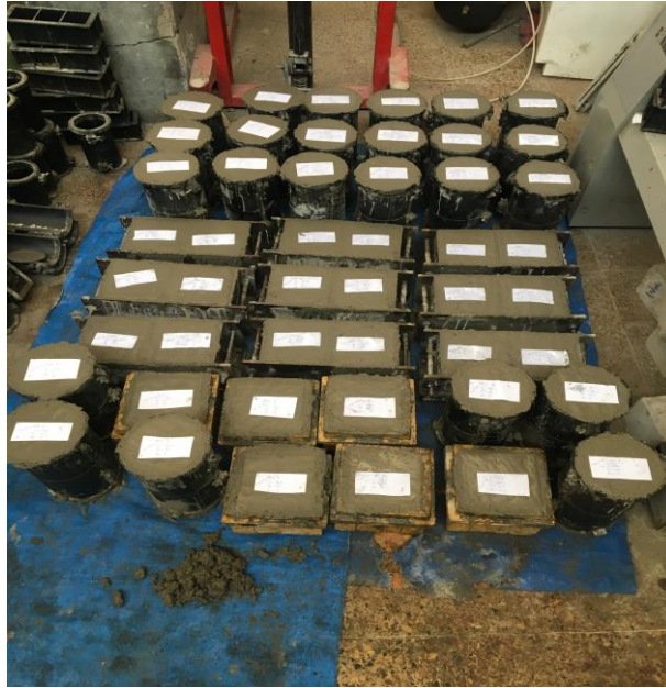
Figure 3.12 Concrete Specimen after cast
