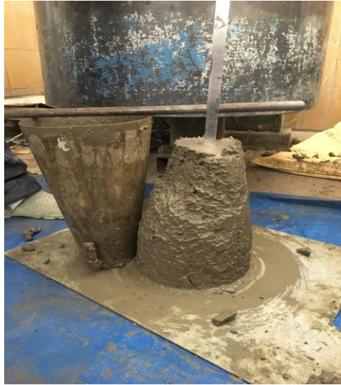
Figure 3.10 Measuring slump of fresh concrete mix
