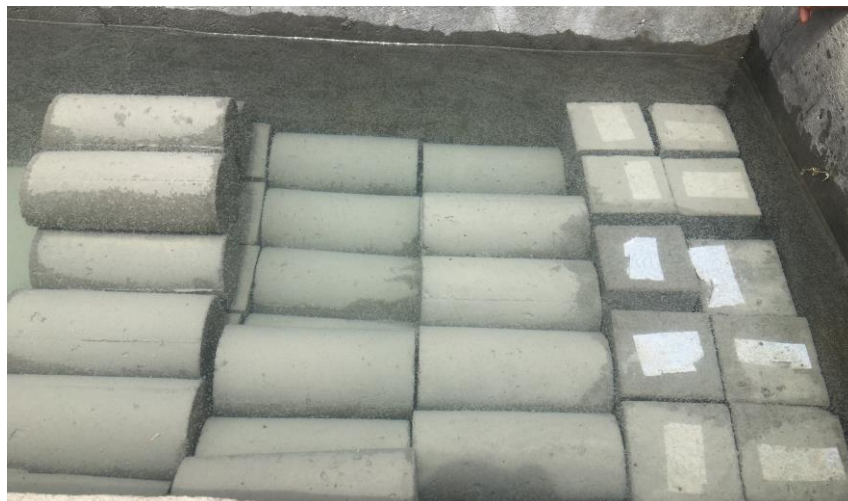
Figure 3.13 Concrete Specimens in water tank for Curing
