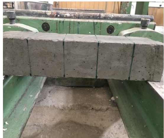
Beam member casted and ready for flexural strength test
