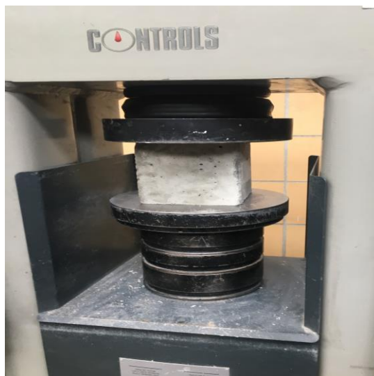
Figure 3.17 Compressive Strength Test Setup
