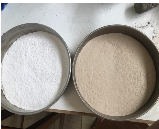
Marble and ceramic waste powders ready for mix
