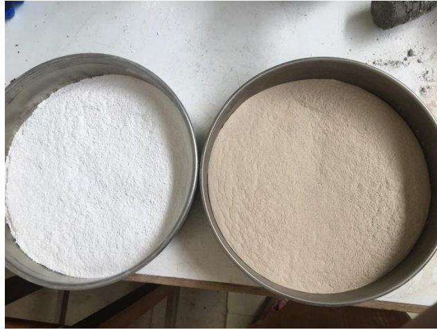
Figure 3.8 Marble and Ceramic powders ready for mix
