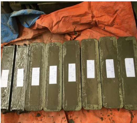
Beam member casted and ready for flexural strength test
