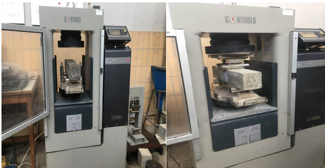
Figure 3.19 Flexural Strength Test Setup
