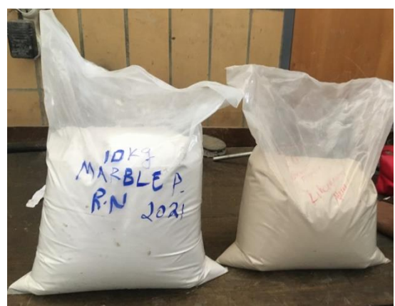
Marble and ceramic waste powders ready for mix
