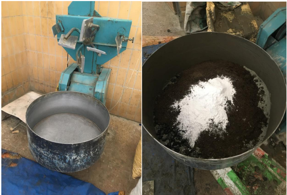
Figure 3.9 Mixer and Ingredients ready for mix
