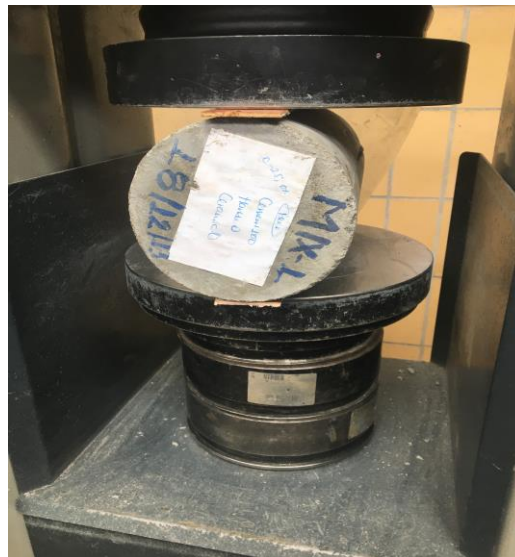
Figure 3.18 Splitting Tensile Strength Test Setup
