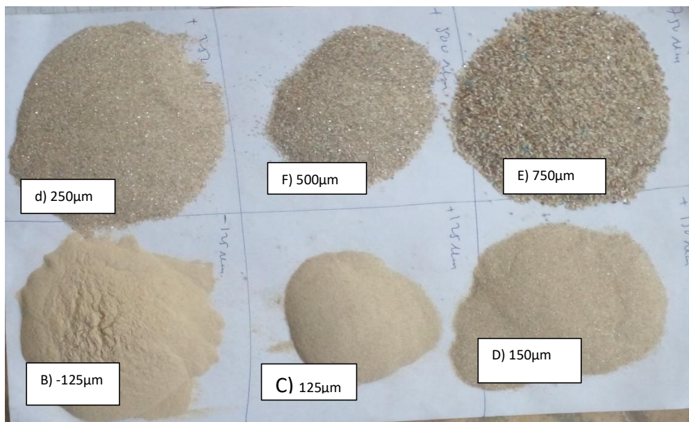
Figure 4.1 PSD after grinding and sieve analysis
