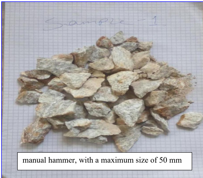
Figure 3.2 Lithium-bearing pegmatite samples after splitting by hammer
