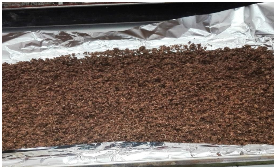
Figure 3.1 Tea waste (Adsorbent) collected and oven dried
