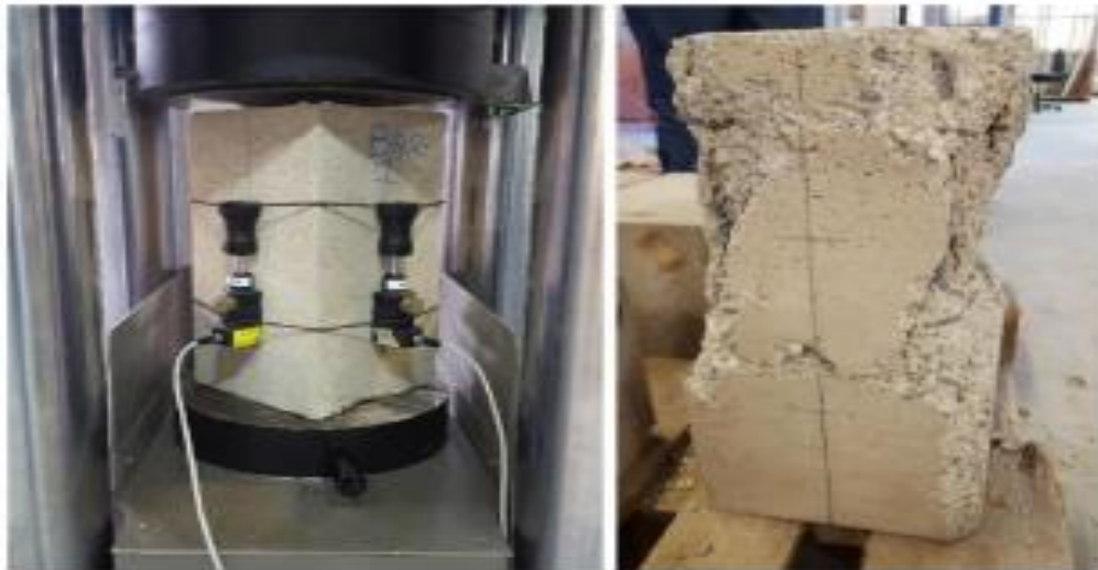
Figure 4. 1 Experimental setup for Compression test on sample of reinforced concrete column [23]
