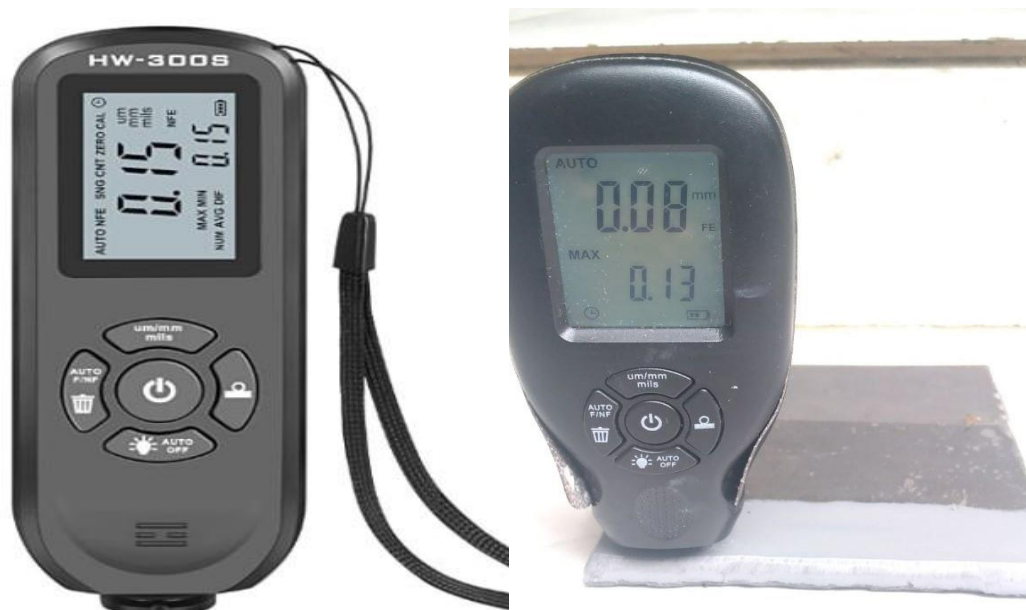
Figure 2: Measuring coating thickness
