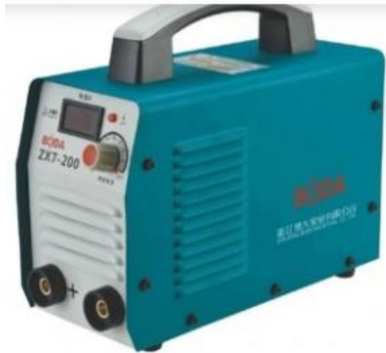
Figure 9: Welding machine used for the experiment(Boda zx7 250 dual voltage 220v/380v manual metal welding machine inverter dc)
