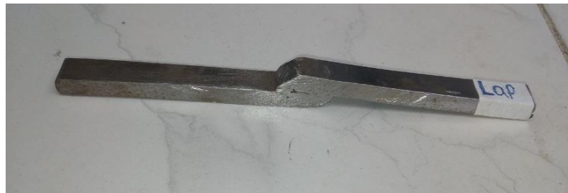
Figure 20: Lap welding sample
