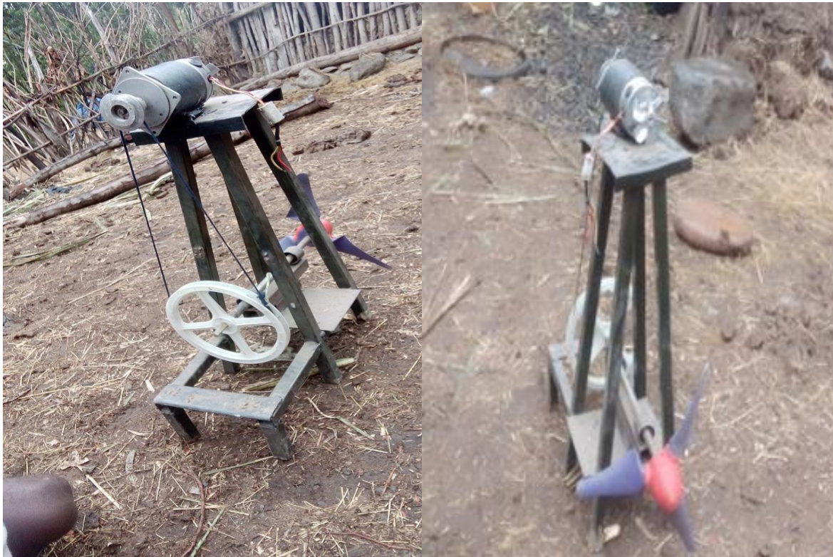
Figure 1 Overall assembly of hydrokinetic turbine
