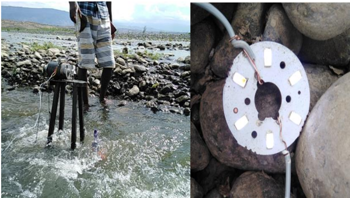
Figure 2 Turbine and bulb during the experiment
