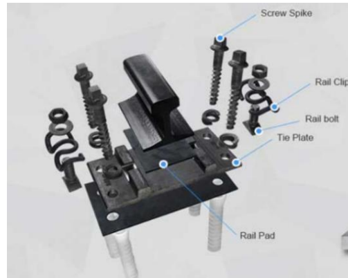
Figure 2-8 Railway fastening system components [71]
