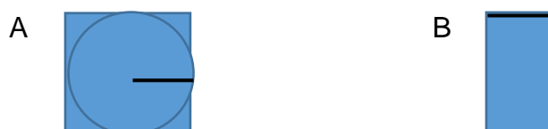
Figure2. 10 (A) Top and quarter section view of 1.1m*1.1m*1.1m concrete block and (B) 1.1 m diameter cylindrical Axisymmetric mass concrete quarter section (simulation by Hacon 3)
