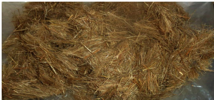
Figure 3-12 Flax fiber ready for surface treatment
