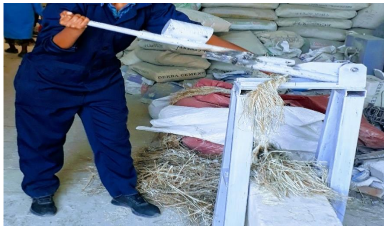
Figure 3-6 Breaking the flax stem by breaker
