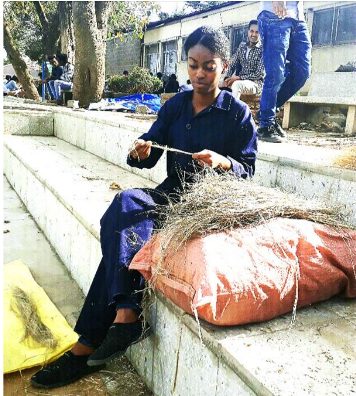
Figure 3-7 Removal of flax shives manually
