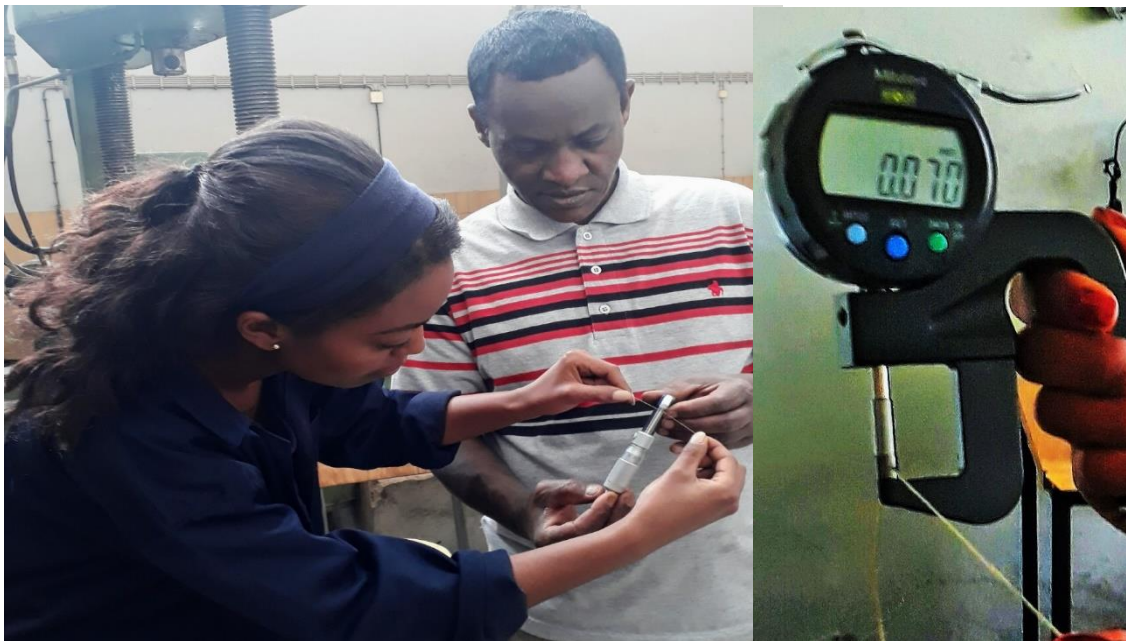
Figure 3-10 Fiber diameter measurement by Micrometer
