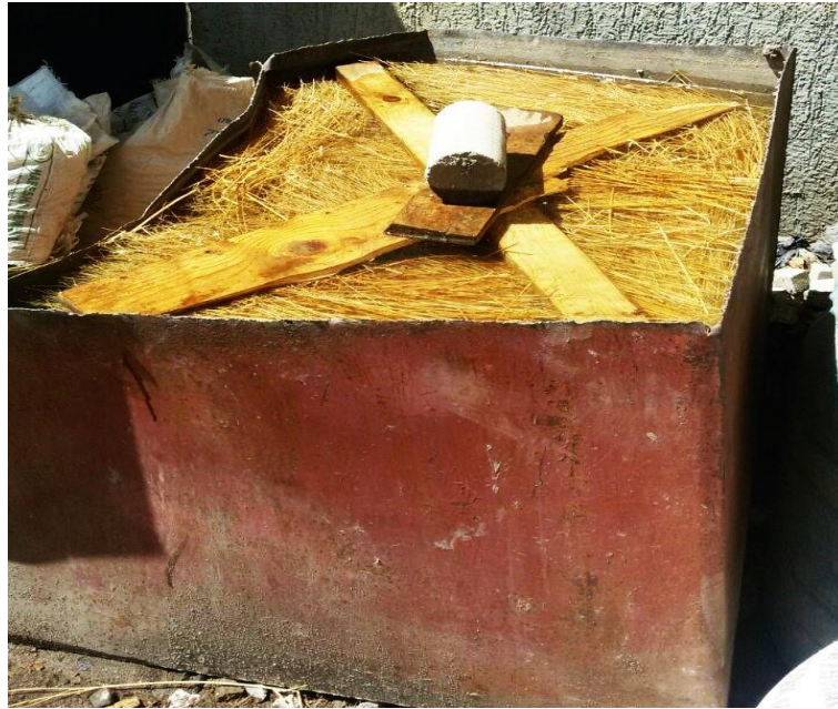
Figure 3-4 Open tank retting of flax stems
