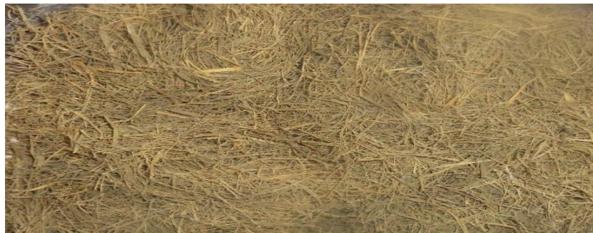
Figure 3-14 Flax fibers coated with cement grout
