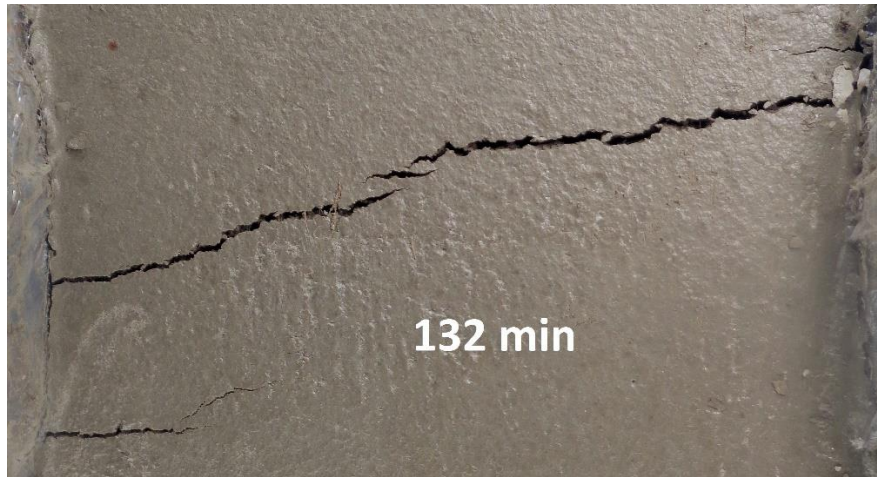
Figure 4-3 Crack initiation and growth in length at 0.0185%
