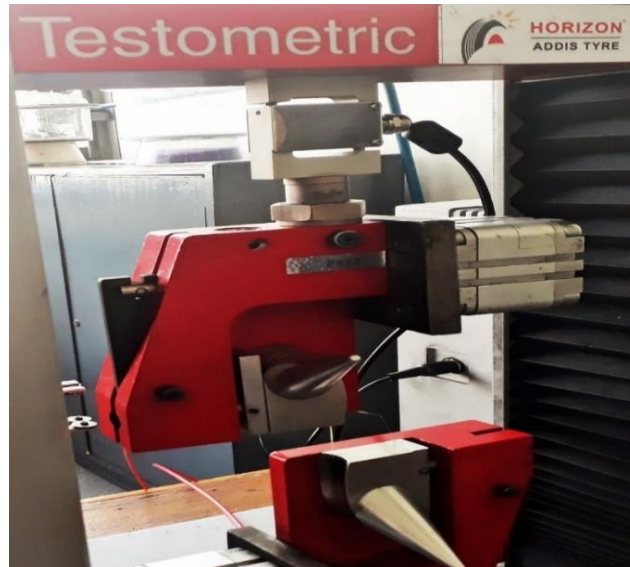
Figure 3-11 Tensile strength test of flax fiber
