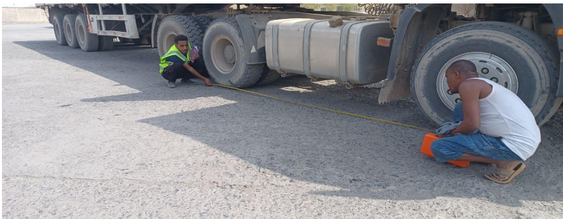
Figure 4-7 Inter-axles spacing sample measurement at Mile Customs Control Station.
