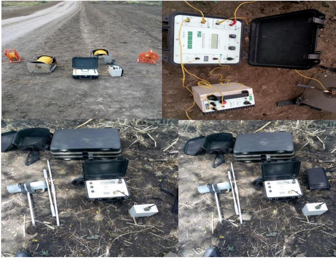
Figure 4.1 Instrumental setup of VES and Magnetic Survey.
