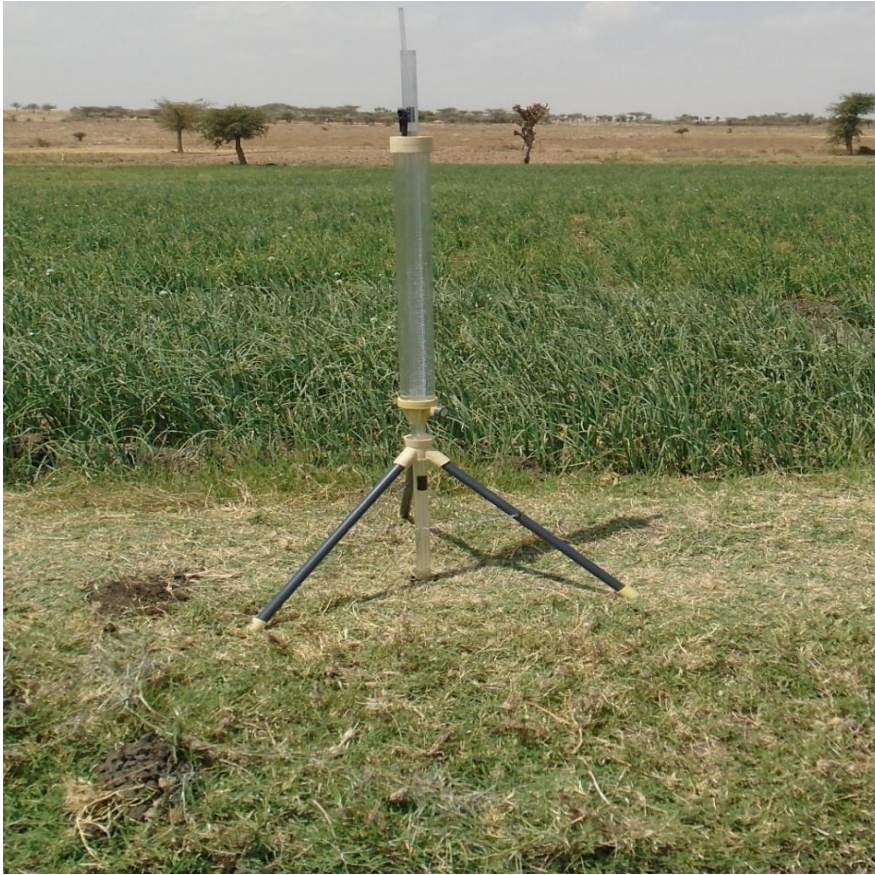
Figure 1.1 Explains measurements of soil field saturated hydraulic conductivity by using Guelph permeameter within the study area.
