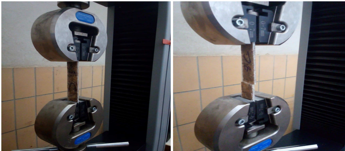
Figure 3. 9 Tensile testing setups and sample after fracture
