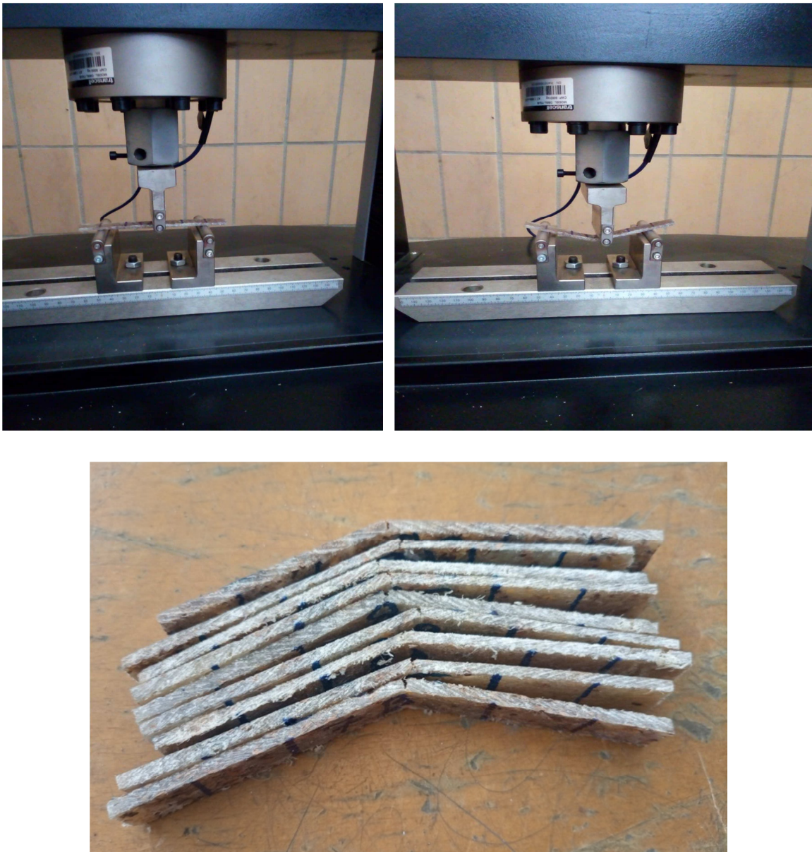
Figure 3. 11 Flexural testing setups and sample after fracture
