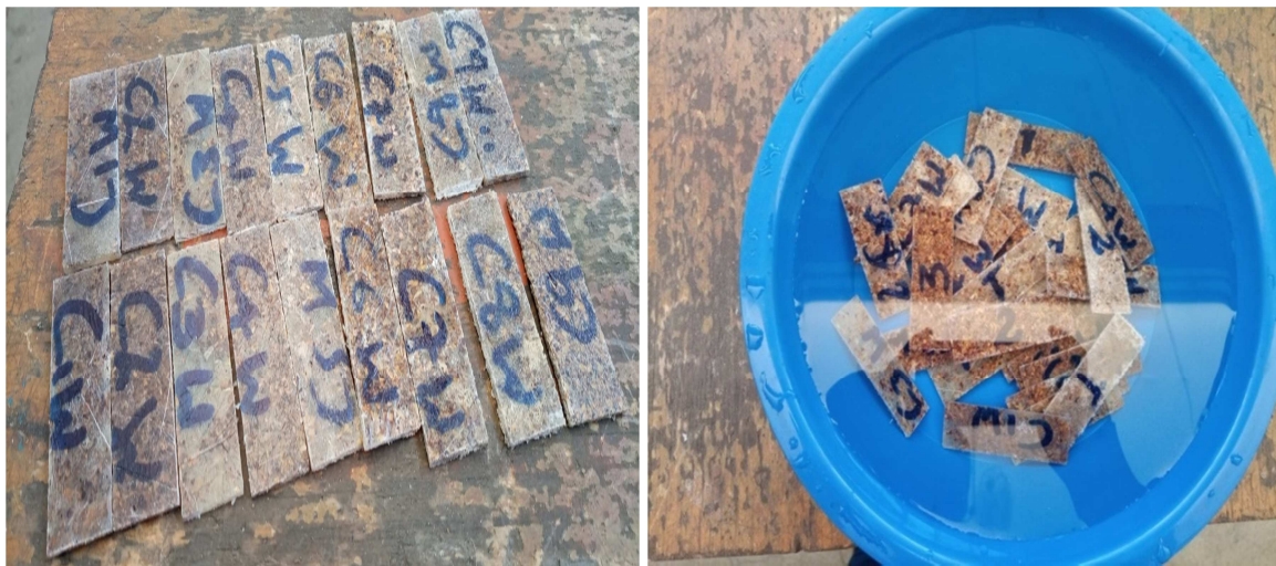
Figure 3. 13 Water absorption specimens submerged in a tank of water
