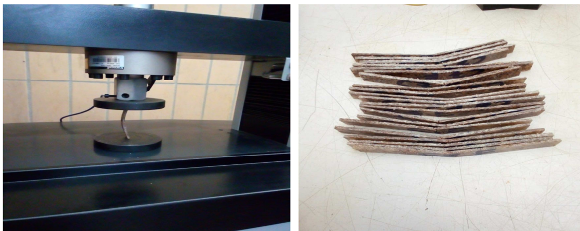
Figure 3. 10 Compression testing setups and samples after fracture
