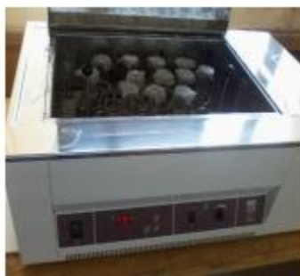
Figure 10 Mixture of Adsorbent and Adsorbate in Thermostat Water Bath Shaker Model No GFL 1083
