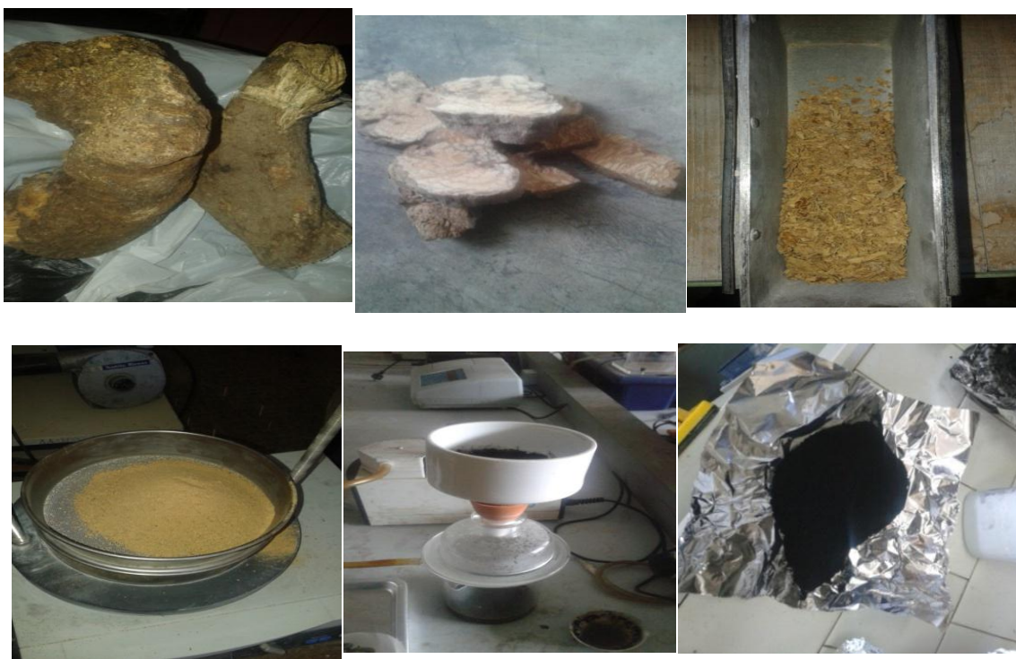
Figure 6 Preparation of Activated Maerua Subcordata
