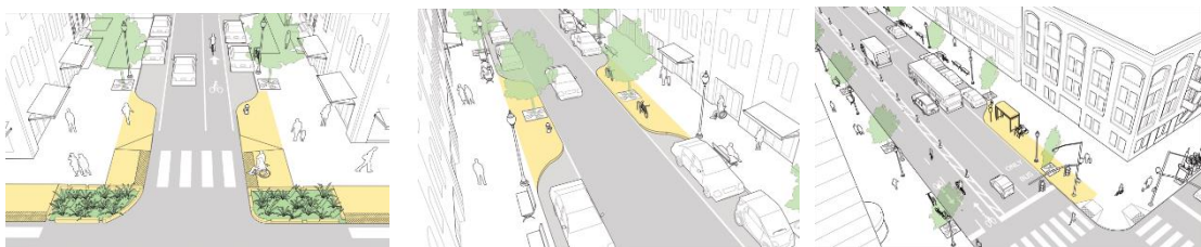
Gateways, bus bulbs, and pinch points: curb extensions that widen sidewalks and could enhance pedestrian safety and comfort. Source: https://nacto.org
