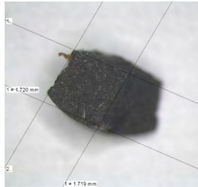
Figure 4.9: Sample photo taken by computerized Camera to measure the dimension for demagnetization factor calculation
