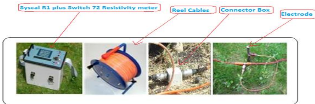
Figure 4.1 Instrumentation of 2D electrical imaging.
