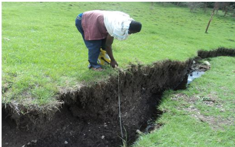
Figure 2.6 Residual clay soils at Shola Wuha locality of the study area showing the deep near vertical fissures.
