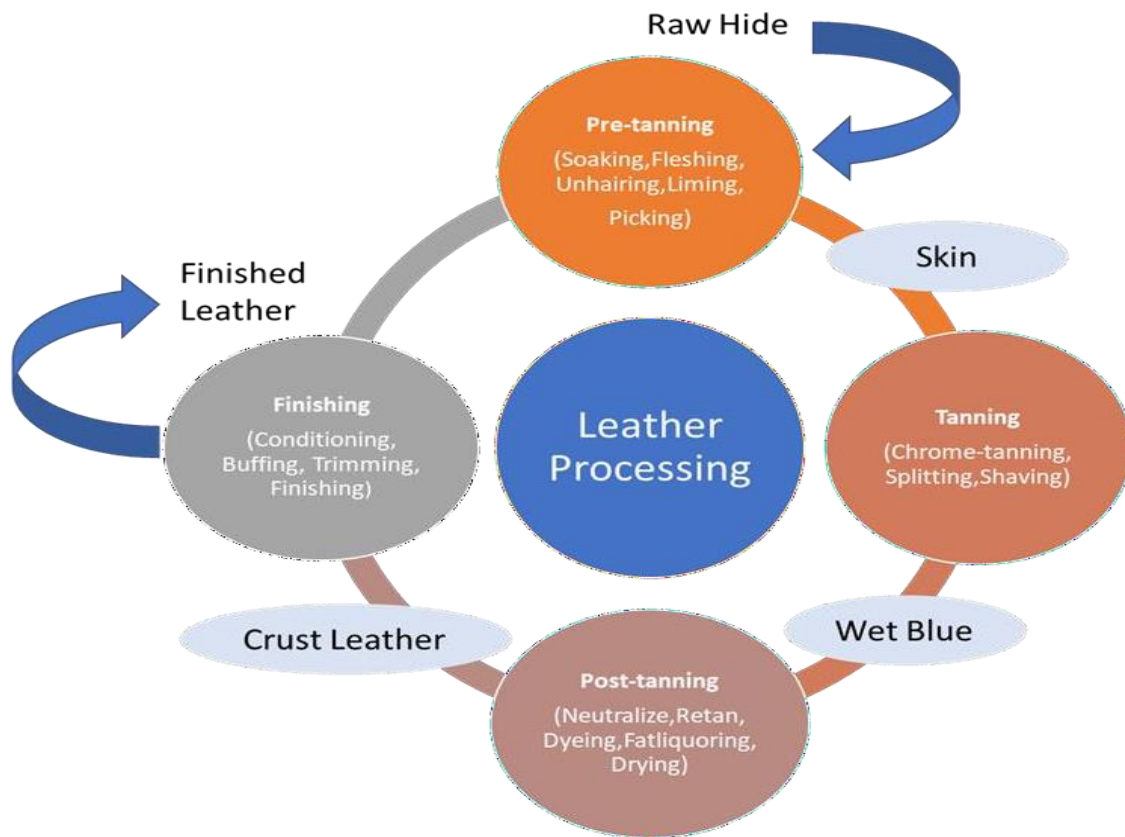
Figure 2-2 Schematic diagram showing general leather processing [38]
