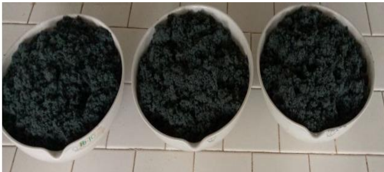
Figure 3-1 Fiberized finished leather waste Fiberized finished leather waste
