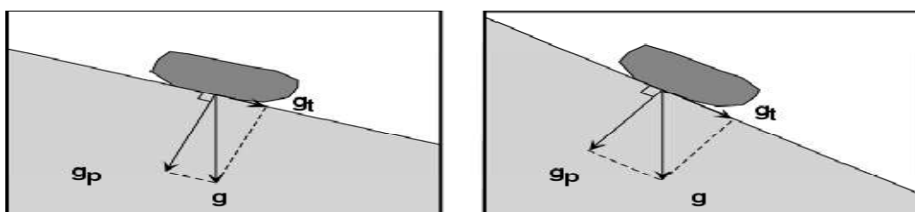
Fig.2. 1 Illustration of tangential components in slope stability analysis (Nelson, 2010)
