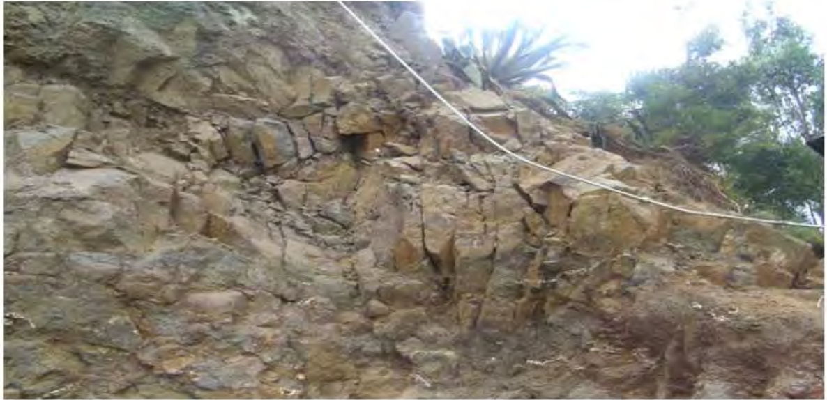
Plate 5.5 Rock mass comprising of Basalt in Mersa town affected by structural discontinuities
