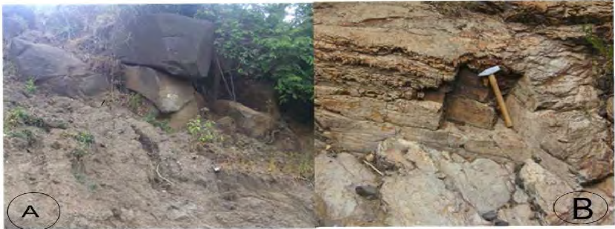
Plate 6.1 Joints dipping parallel to the slopes (A) Mersa & (B) Wurgessa
