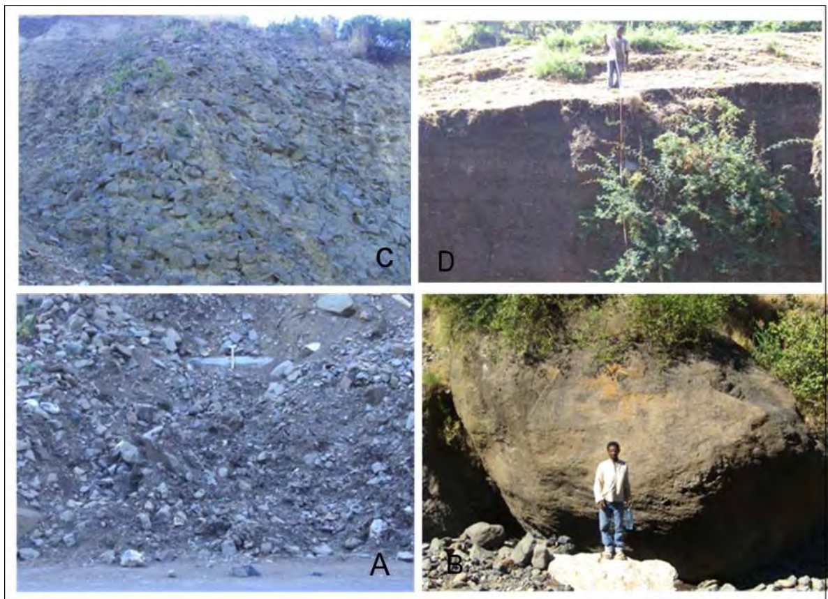
Plate 5.2 (A) Colluvial material slide with rock fragments of sharp edge. (B) Boulder slide at the foot of the slope (C) Loose rock fragments (D) Alluvial deposits (Wurgessa)
