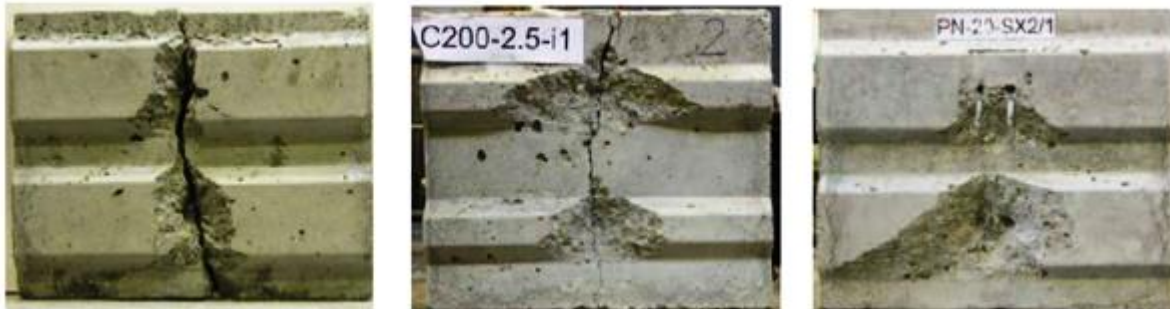
Figure 13 Characters of concrete failures in composite connections
