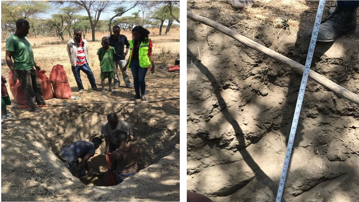
Picture 4. 1: Collapsible soil samples collected from the test pit
