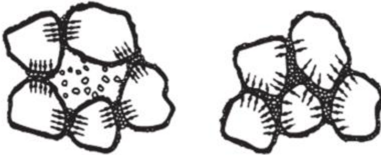
Figure 2. 3: a) Dry soil with honeycombed structure before inundation (b) Soil structure after inundation
