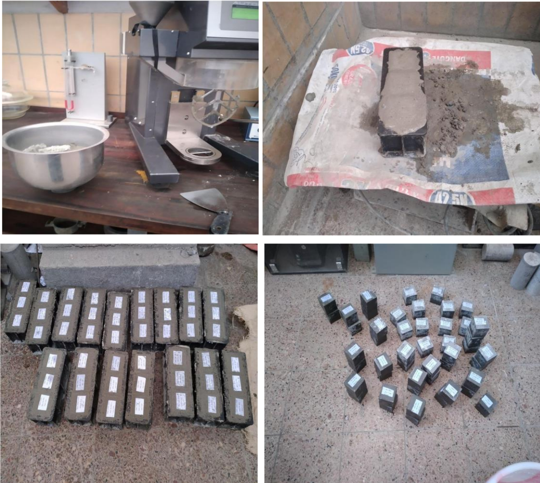
Figure 3. 7 shows the mixing, vibrating, moulding and demoulding of the specimen
