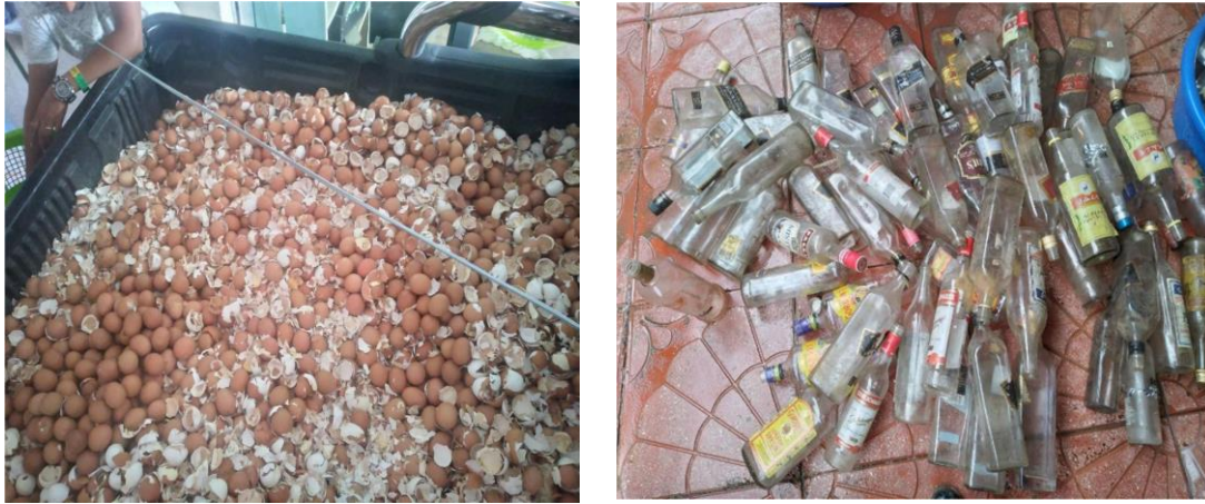
Figure 3. 1 Samples of egg shell and waste soda lime glass used for cement replacement
