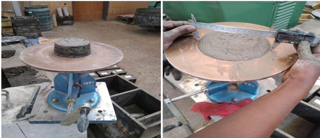
Figure 3. 9 Flow test conducted for the given sample
